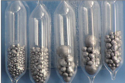
Fig. 1: Granules of pure Silicon enclosed in ampoules made of highly pure silica.
