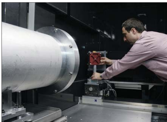
Preparing a fuel cell for tomographic imaging
