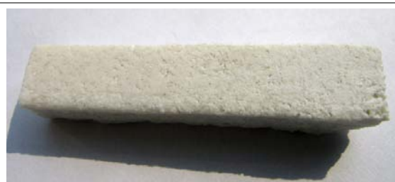
Fig. 1: Nano-scale refractory analogue: Alumina and zirconia nanoparticles embedded in a sodium / potassium silicate glass matrix.
