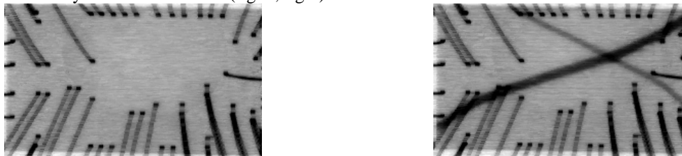
Fig. 3: Radiograph of the bonding wires, (left) without and (right) with dark bands, respectively
