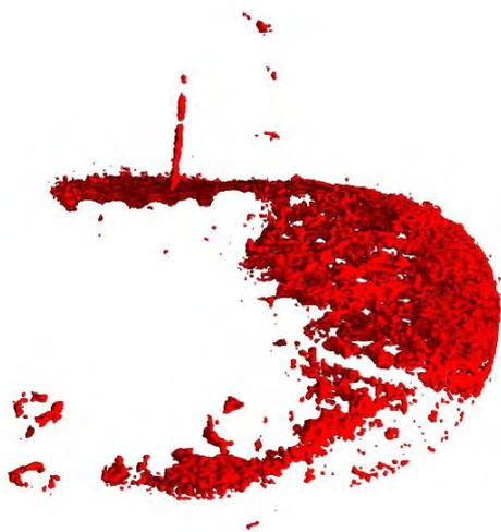
Figure 8: Visualization of the main fatigue crack of the LCF sample without matrix and fibres. The scattering plane of the analysing crystal was parallel to the fibre direction.
