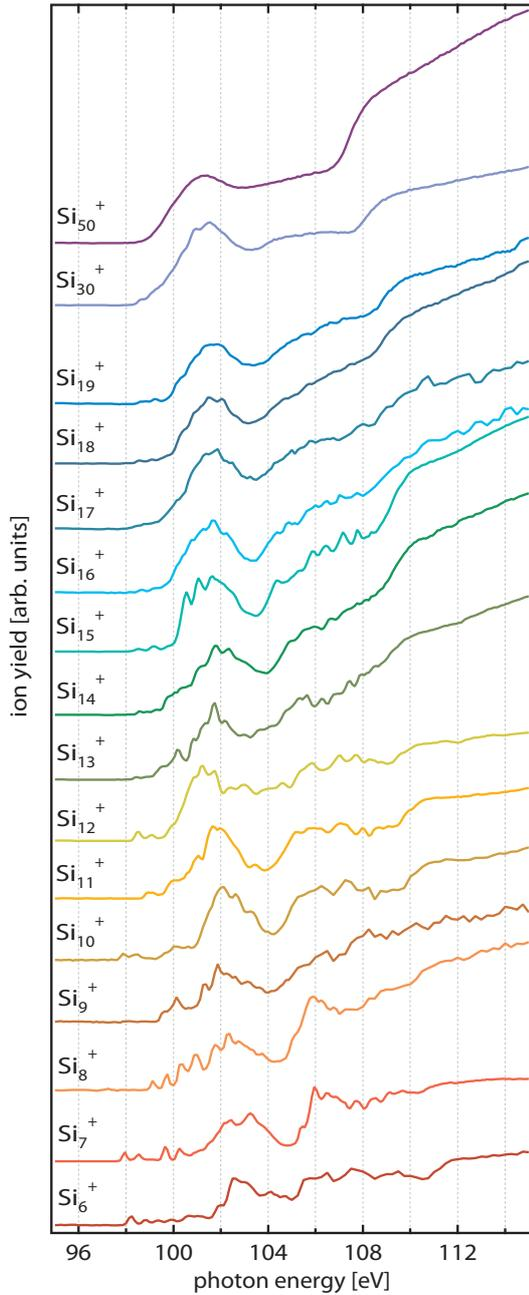
FIG. 1: Total ion yield spectra of  $Si_n^+$  for  $n = 6 - 50$ .
