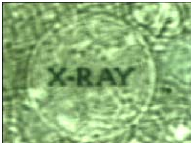
Figure 3. The image reconstructed from the synthetic hologram.
