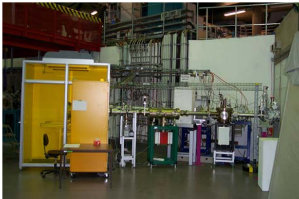
EUV beam line: pre-mirror chamber on the right, multilayer mirror chamber in the middle, clean room hutch with exposure station on the left
