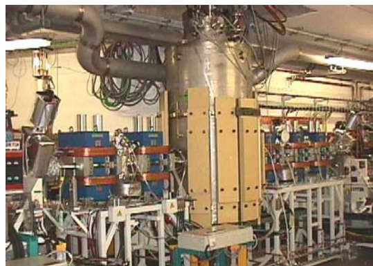
Fig. 7: Photo of the 6 T WLS, formerly operated at BESSY I, that replaced the 4 T device
