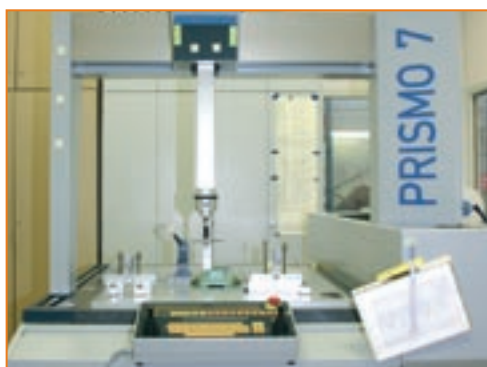
Fig. 2: Using a 3D coordinate measuring machine (PRISMO 7, Zeiss) mechanical tolerances in the range of a few microns are determined. The BESSY system additionally allows for a geometric correlation of part size and magnetic field.
