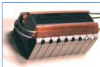
Fig. 7: Optical element in its holder with additional cooling plates attached
