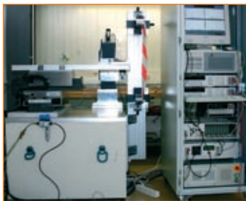
Fig. 1: High precision test stand for single magnet block characterization. By moving a magnetic block with respect to a stretched out wire (mimicking the electron beam) the induced voltage is representative for the integrated magnetic field.
