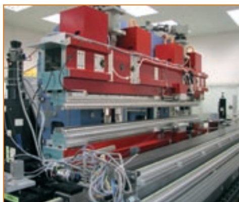
Fig. 6: Precision bench for local field measurements and shimming
