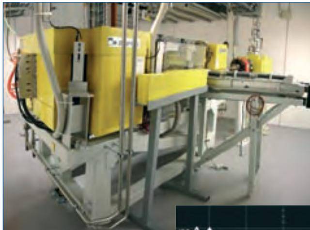
**Fig. 10:** 100 MeV injection microtron installed in the microtron bunker. The inlay shows a measurement of the current pulses of the microtron at two positions in the transfer line during commissioning. The specified value of 8 mA for the current pulses is even exceeded.
