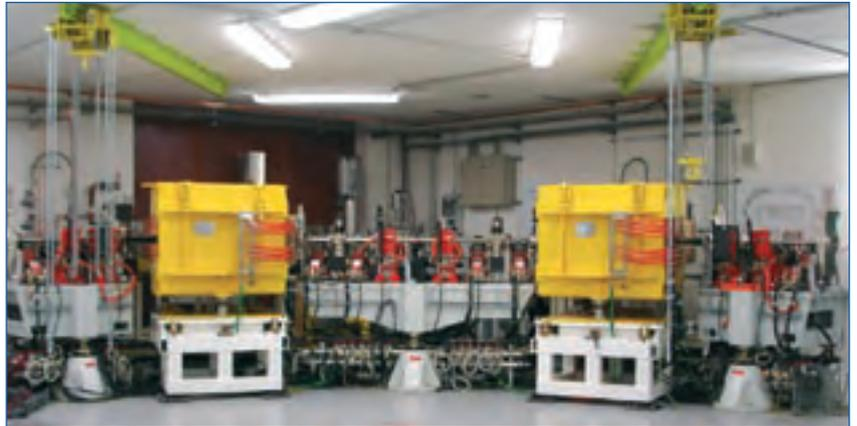
**Fig. 9:** One of four magnet sections with the vacuum chamber system installed. The upper part of the multipole magnets has been removed for the vacuum chamber installation.
