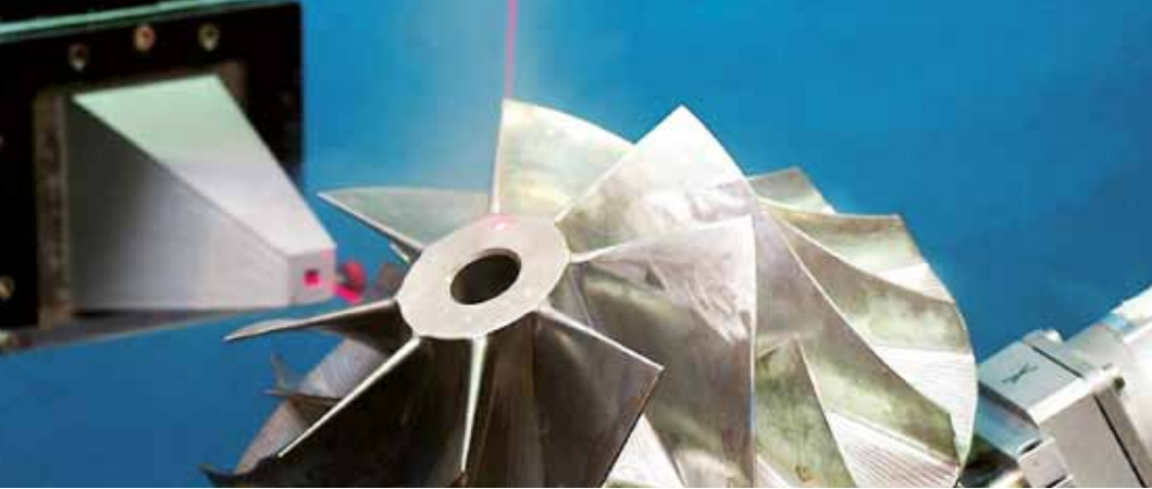
A compressor turbine prepared for non-destructive evaluation of stress states using neutron diffraction method.
