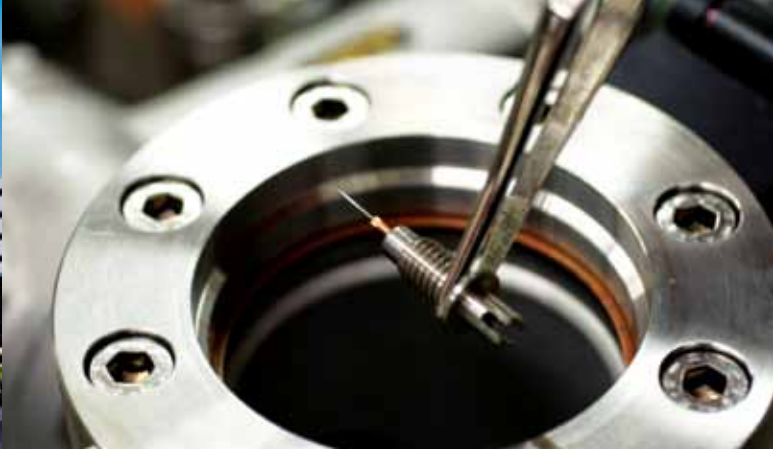
Specimens in the form of a fine needle are used for investigations at the three-dimensional atom probe. This instrument permits the elemental reconstruction of a small volume of metallic material with near atomic resolution.
