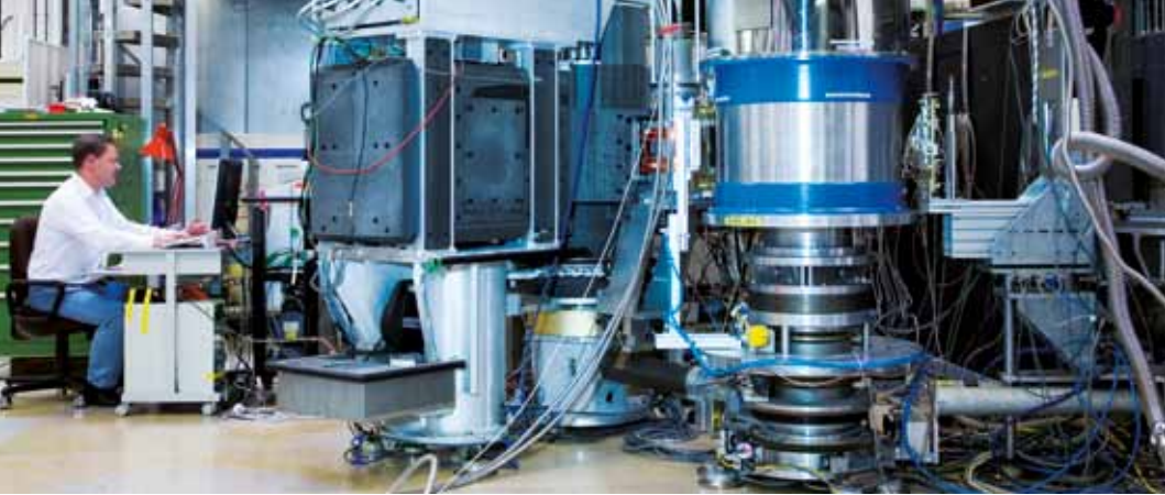
3-Axis Spectrometer FLEX with high field sample environment. Most experiments on high temperature superconductivity are done here.
