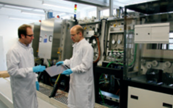
Employees are testing a new coating option at the PVcomB's sputter facility.
