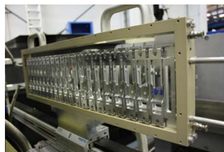
20-Position sample changer, windows temperature controlled, removable
