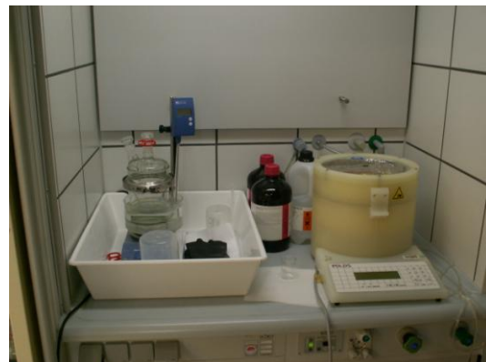
Extractor hood equipped with high speed spin coater (right) and wet etching tools (left).
