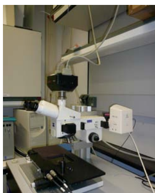
Left: Fluorescence microscope with spot illumination
