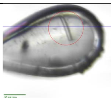
11 \mu\text{m} crystal within a 50 \mu\text{m} X-ray beam
