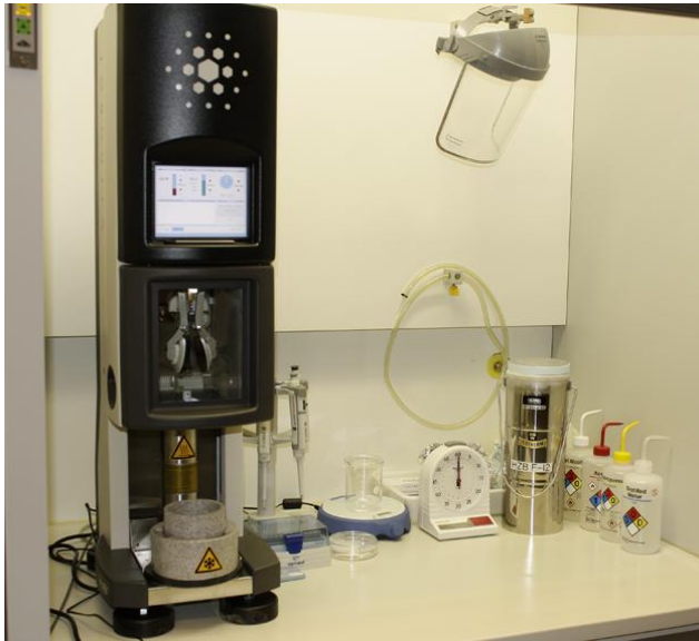
Automated plunge freezing device (FEI Vitrobot™) for vitrifying particles in the liquid dispersed state. © Polzer
