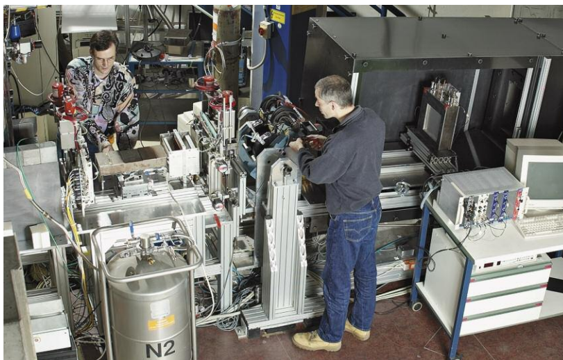
With the reflectometer (V6) at the neutron source BER II, the scientists gained insights into the structure of the magnesium alloys.
