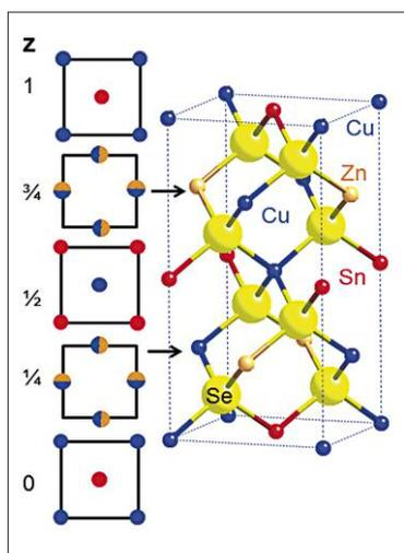
Picture of a kesterite structure containing selenium (yellow), copper (blue), zinc (orange) and tin (red).
