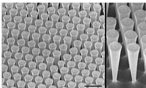
Scanning electron micrographs (SEM) show how regularly the funnels etched in a silicon substrate are arranged (left: the line segment = 5 microns; right: 1 micron). The funnels measure about 800 nanometres in diameter above and taper down to about a hundred nanometres at the tip.
