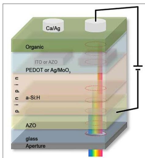
The a-Si:H is deposited on an AZO film that acts as a transparent front contact. An ITO layer serves as rear contact. The organic sub-cell possesses a front contact made of a conductive polymer material (PEDOT) and a metallic rear contact.
