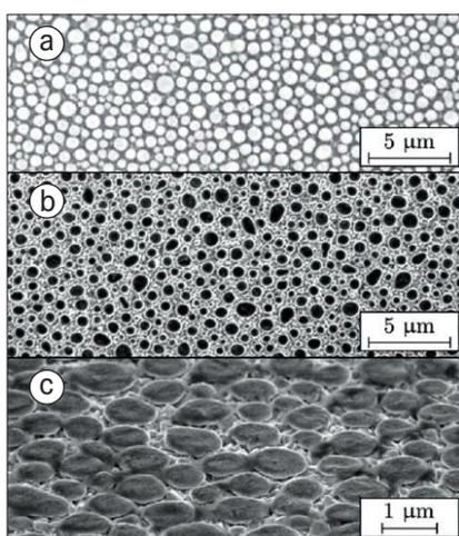
Ammonium tungstate/PSS film surface: (a) SEM image before pyrolysis; (b & c) SEM image after pyrolysis.
