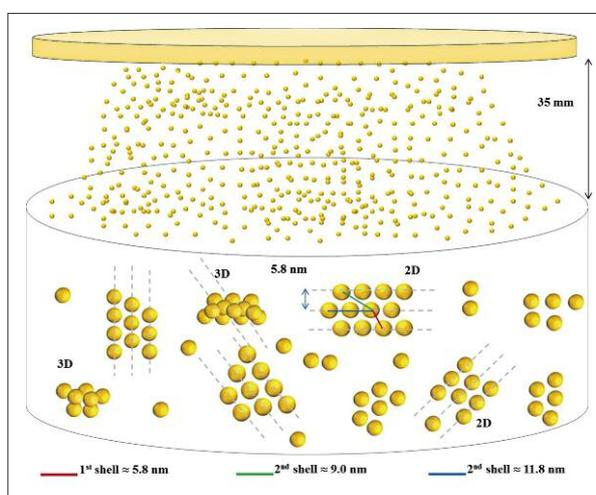
Model of the self-assembly mechanism of clusters of gold nanoparticles.
