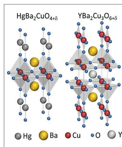
Crystal structures of  $\text{HgBa}_2\text{CuO}_{4+\delta}$  and  $\text{YBa}_2\text{Cu}_3\text{O}_{6+\delta}$ .
