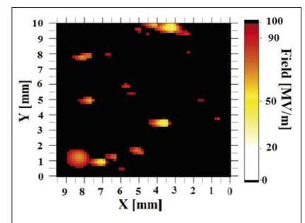
Field emission maps of an annealed oxide-free (top) and thermally oxidized Mo surface (bottom). The oxide apparently reduces the number of emitters providing 1 nA of current at fields of up to 100 MV/m.
