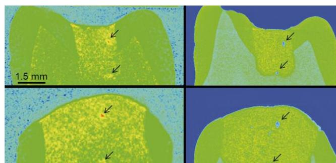
The neutron images (left row) detect the distribution of liquids in this filled tooth, whereas the X-ray-CT shows the microstructure and pores in the material. A comparison of both images shows which pores are filled with liquids.
