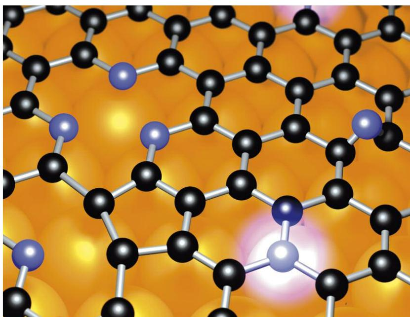
Graphene populated with different nitrogen impurities (blue atoms). The underlying gold surface promotes the controllable conversion of impurity-related defects into substitutions (glowing atoms), which effectively donate electrons to N-graphene.
