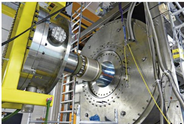
Insertion of the resistive Bitter coil into the superconducting coil. These strong copper lines provide current.
