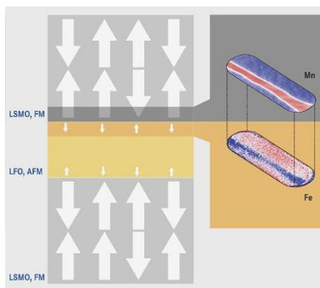
The insulating LFO-layer in its normal state is antiferromagnetically ordered (AFM) and has no ferromagnetic domains. Due to the proximity to the ferromagnetic LSMO, ferromagnetic domains develop (white arrows) at the interface, pointing into the opposite direction of the LSMO-layer.
