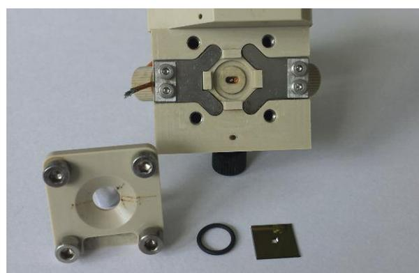
In the new measuring cell of the LiXEdrom, electrochemical reactions at the interfaces between solids and liquids can now be studied in a vacuum with soft X-rays.
