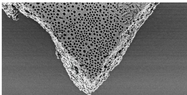
A talent for motion: thanks to its pores and chemical structure, the biomimetic membrane developed by the scientists from the Max Planck Institute of Colloids and Interfaces curls faster and more vigorously than comparable materials.
