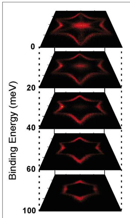
Both figures display experimental data on the “Dirac cone”. The outward warping is pronounced as well as the broadening of the boundaries of the cone which is caused by collisions of the electrons with obstructions in the real, non-ideal, topological insulator bismuth telluride.
