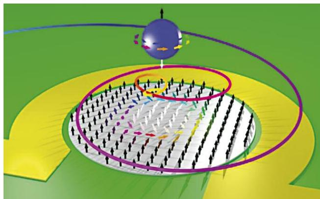
The local magnetisation is depicted by small arrows; a magnetic vortex is located in the centre. A brief current pulse through this nano-wire deflects the skyrmion out of its rest position; it then moves back to its initial position on a spiral trajectory. This motion can be observed with the help of X-ray holography. The skyrmion and the spiral shape of its trajectory are represented schematically above the structure.
