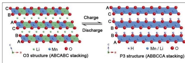
The original structure of the material has an ABCABC arrangement of oxygen layers (left). Due to the  $\text{Li}+\text{H}+$  exchange during the charging process it degrades to ABBCCA (right).
