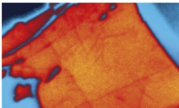
The sample consists of a layer of tungsten selenide (orange) applied to a layer of molybdenum sulphide (blue). Studies with the SPEEM microscope at BESSY II show that energy transfers between the two semiconductor layers yields an electric potential of up to 400 meV.
