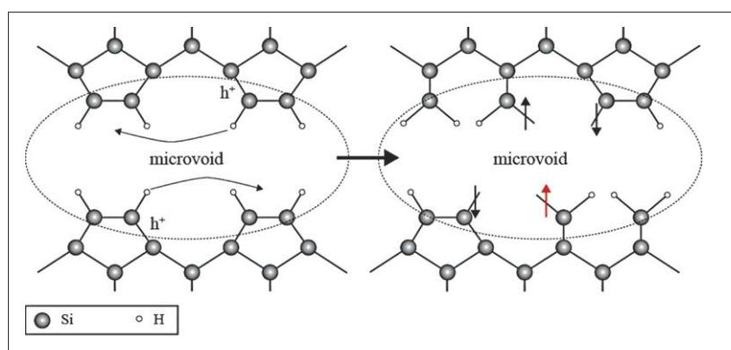
In the initial state (left), the voids' internal surfaces are saturated with hydrogen atoms so that no defects are observed. Light-induced charge carriers ( $h^+$ ) destabilize atomic bonds. The breaking of atomic bonds causes defects (indicated by the vertical arrows on the right-hand side), which translates to reduced solar cell efficiency.
