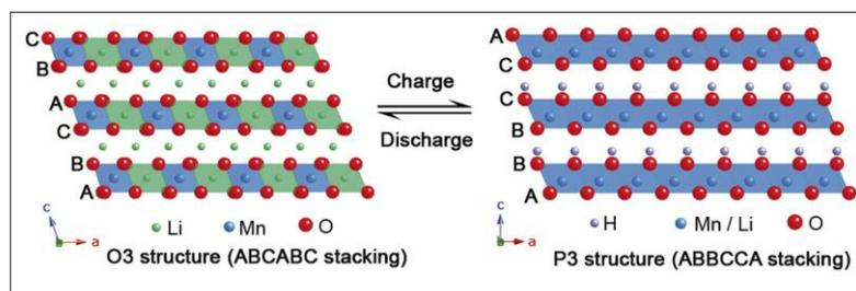
The original structure of the material has an ABCABC arrangement of oxygen layers (left). Due to the  $\text{Li}+\text{H}+$  exchange during the charging process it degrades to ABBCCA (right).
