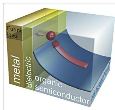
When inserting an ultrathin dielectric between metal electrode and organic semiconductor, charge carriers (shown here for a positively charged hole in red) are, counter-intuitively, more efficiently extracted from their transport level (blue) in the organic to the Fermi level (black) in the metal than without the interlayer.
