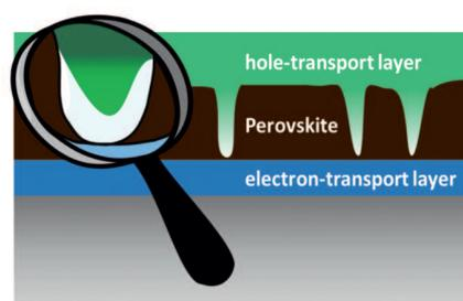
Simplified cross-section of a perovskite solar cell: the perovskite layer does not cover the entire surface, but instead exhibits pinholes. The scientists showed that a protective layer builds up, preventing short-circuits.
