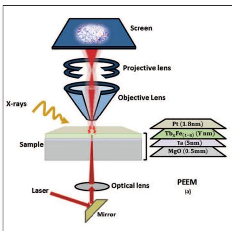
A research team led by Kronast empirically established that the warming of the storage material by the energy of the laser light plays an instrumental role when toggling the magnetisation alignments, and that the change in the material only takes place under certain conditions.
