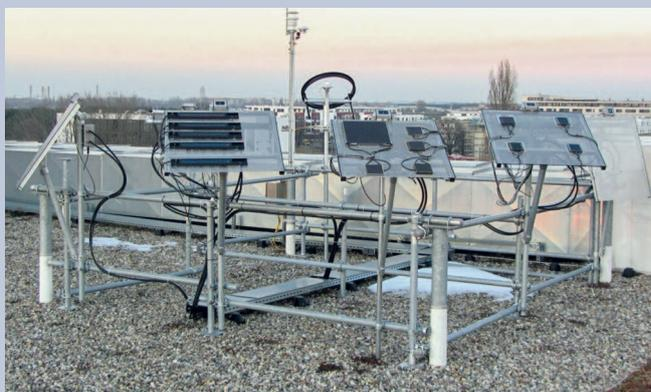
The energy yields of CIGS modules under real-world conditions can be measured on an outdoor testing platform at PVcomB.
