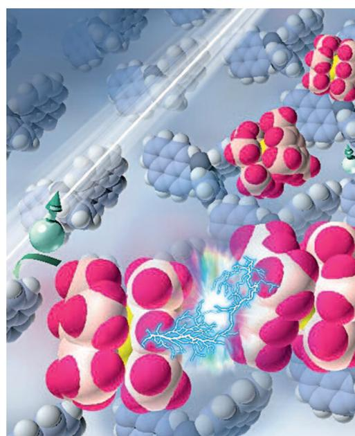
The illustration shows how photons break the dimers into the individual organometallic molecules again, which then effectively n-dope the organic semiconductor.
