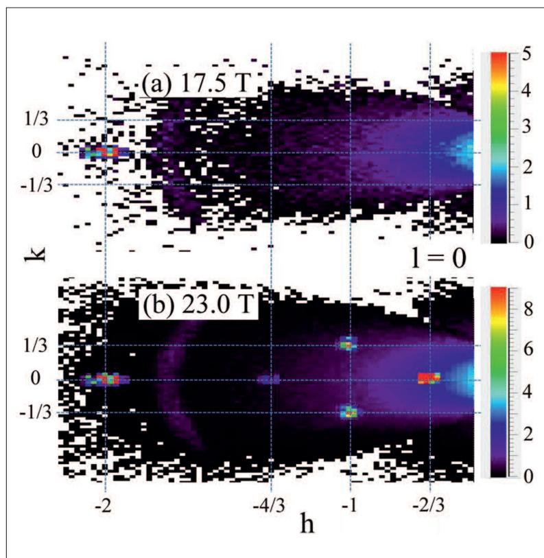
Additional spots appear on the neutron detector starting at a magnetic field strength of 23 teslas, revealing the new magnetic order in the crystal.
