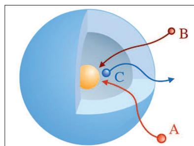
Sketch of a yolk-and-shell-type nanoreactor: reactants A and B diffuse through the shell and react to form C at the catalytically active nanoparticle (yellow).
