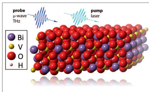
Using time-resolved conductivity measurements in hydrogen-treated bismuth vanadate ( $\text{BiVO}_4$ ), researchers have shown that electrons and holes last twice as long in this material. This increases the material's efficiency as a photoelectrode.
