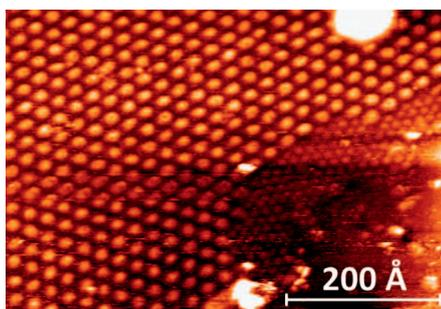
electrons extremely well. Surprisingly, if you apply a layer of graphene to a nickel substrate and shove atoms of gold in between, then what is known as the spin-orbit interaction dramatically increases by a factor of 10,000, allowing the orientation of the spins to be influenced by external fields.
