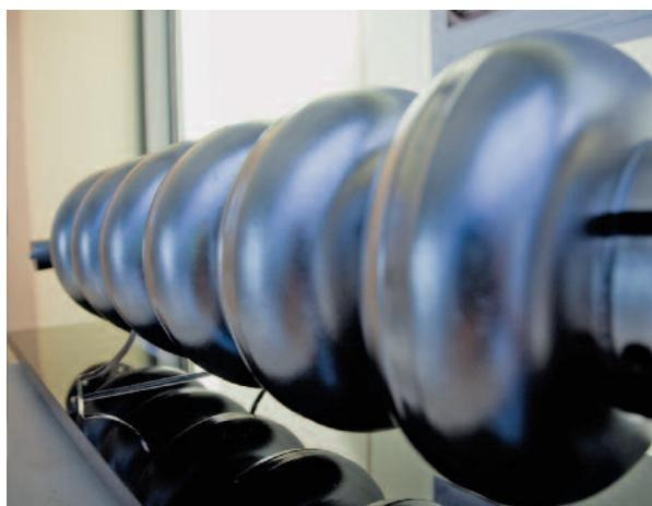
A model of the linear accelerator (linac) with superconducting cavities.
