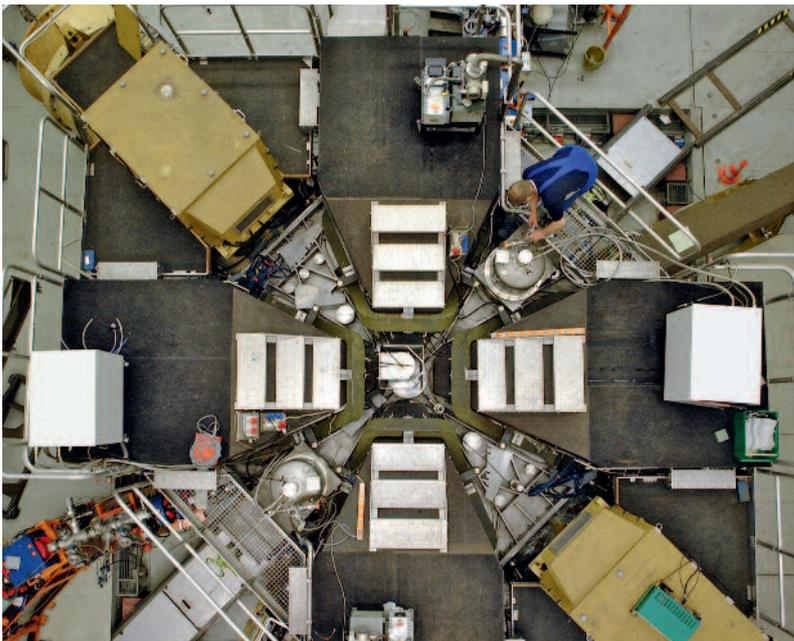
The Cyclotron of Helmholtz-Zentrum Berlin is part of the particle accelerator that delivers the proton beam for eye tumour therapy.
