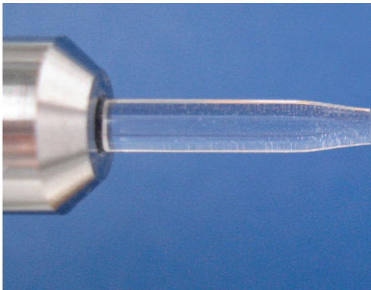
Close-up of the liquid jet from which the stream of liquid sample shoots in front of X-rays at a speed of 288 kilometres per hour.
