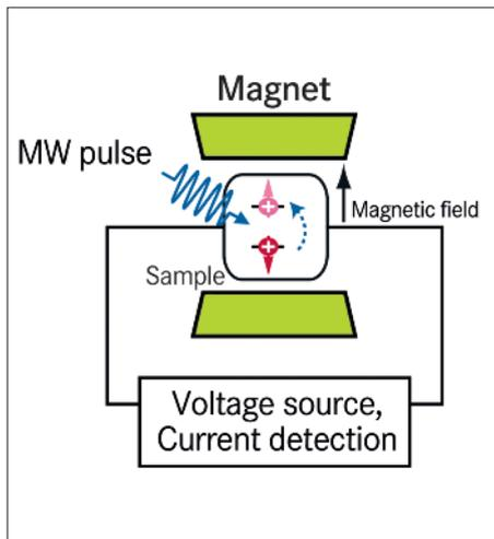
Principle of EDMR (electrically detected magnetic resonance): The sample is irradiated with microwaves and simultaneously exposed to a strong magnetic field.
