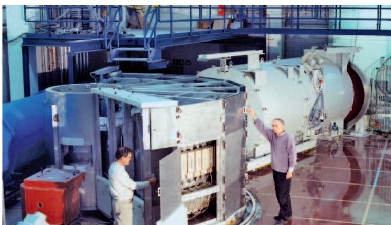
The time-of-flight spectrometer is being rebuilt and housed in an extension.
