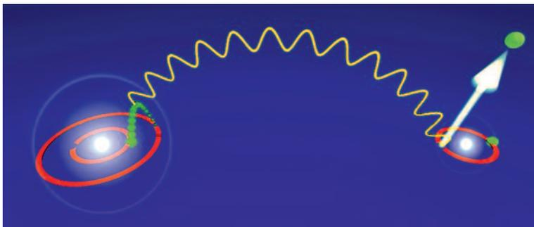
In a helium dimer, consisting of two helium atoms, one of the atoms (left) is excited by a photon. This produces a new photon whose energy (yellow line) is transferred to the second atom (right). There, it knocks out an electron (green).
