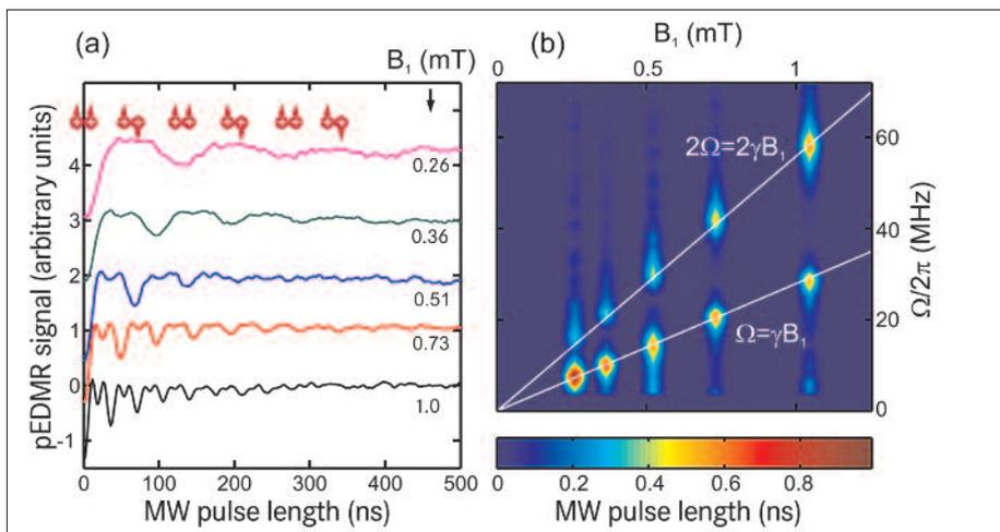
Characteristic fluctuations show up in the EDMR signal as a function of pulse length, indicating a polaron pair with spins oriented in parallel or antiparallel.
