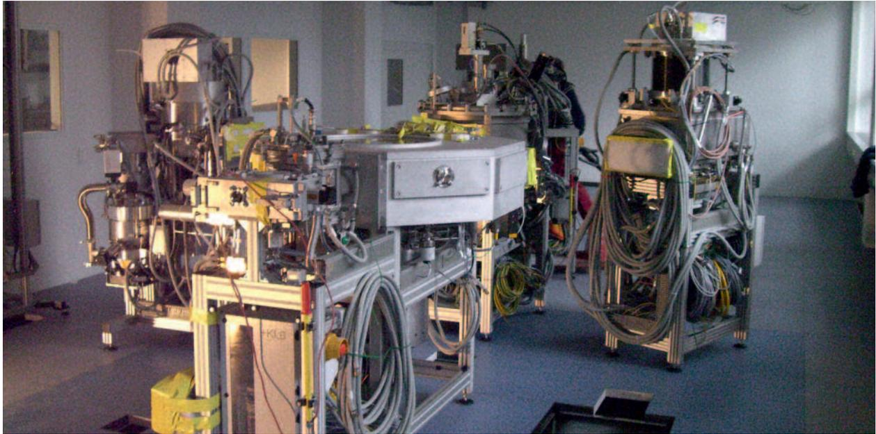
The new cluster tool of PVcomB is now in operation. HZB scientists have already produced the first large-format photovoltaic modules on this research line.
