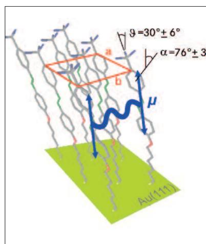
Geometric illustration of azobenzene alkanethiol: the orientation of the molecules (angles “alpha” and “theta”) were measured to estimate the influence of the excitonic coupling on the switching behaviour of azobenzene in densely packed SAMs.
