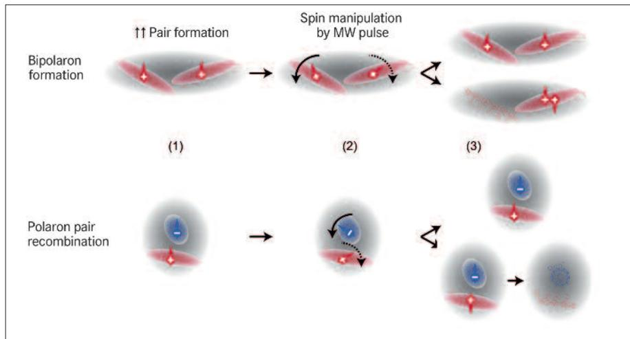
Using synchrotron radiation and EDMR, researchers manipulate the electron spin of the current-carrying particles (polarons). The spin can be turned like a compass needle. Measurements reveal that current flows freely when the tiny magnets are oppositely aligned. When aligned in the same direction, the flow of current is blocked.
