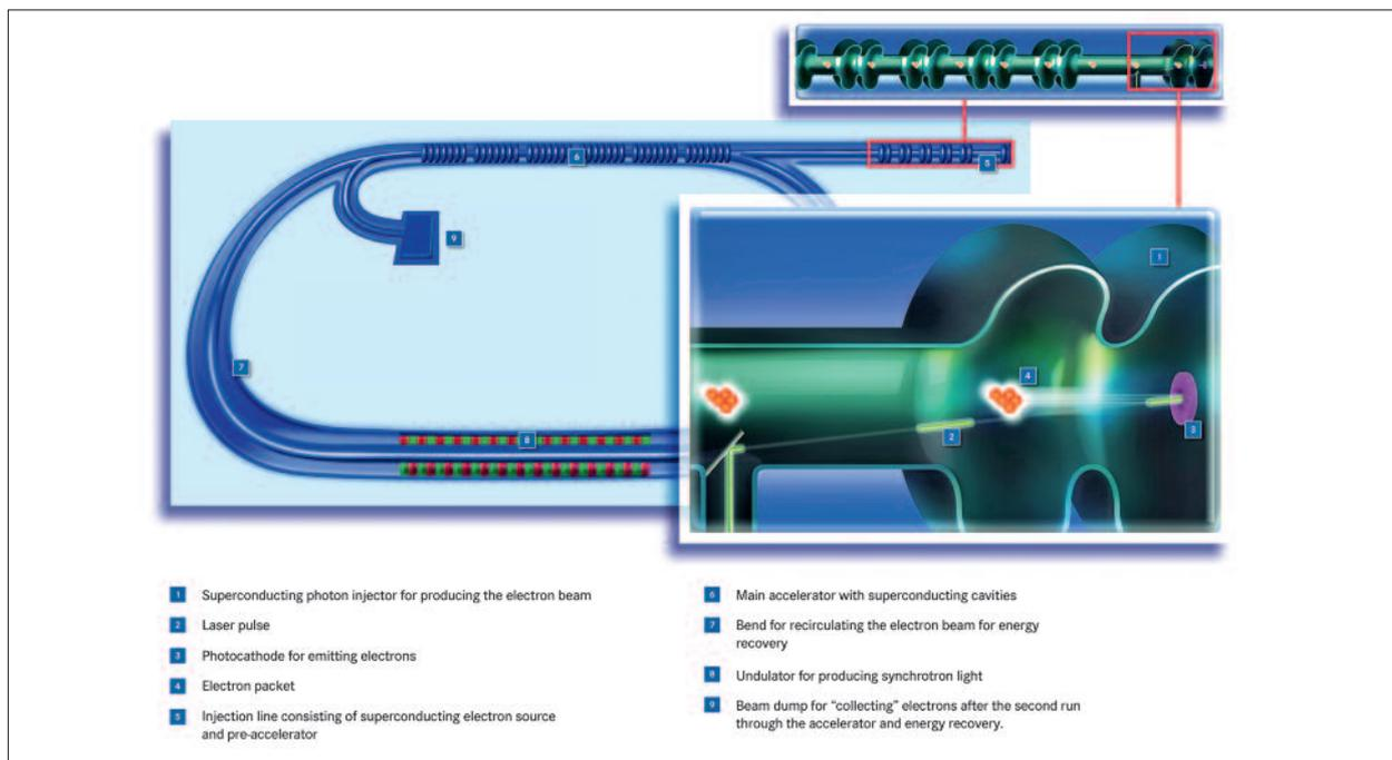
In the energy recovery linac prototype (BERLinPro), electron packets are generated in the injector and accelerated in a long, straight and superconducting linear accelerator (linac) before being guided through magnets where they produce X-rays as in a synchrotron radiation source.
