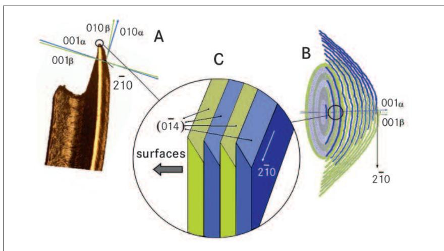
Only under the high-resolution X-ray beam from BESSY II does the sea urchin tooth (A) reveal its secret: It consists of staggered crystal layers (C) that overlap at the tips (B). Even with abrasion, they always stay sharp.
