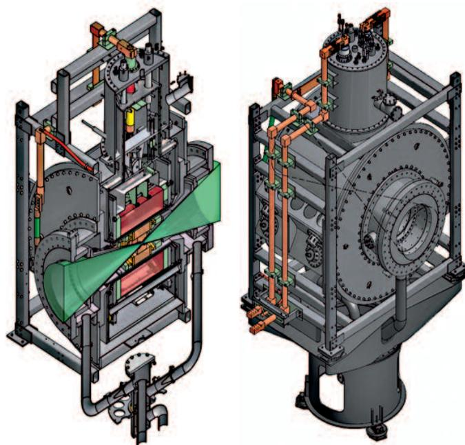
Cross-section of the high field magnets: The neutron experiments take place inside the magnetic cone.
