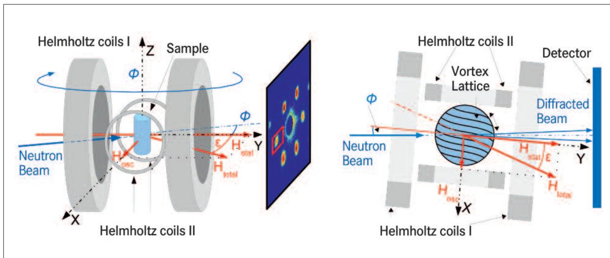
To measure the dynamics of the flux lattice in the niobium crystal, the sample (pale blue) was subject to two crossed magnetic fields (grey rings) while being bombarded with neutrons. By changing the orientation of the magnetic field, the intensity of the neutron scattering also changes. With these measurements, the scientists gained precise insights into the arrangement of the flux tubes inside the niobium crystal at extremely low temperatures.
