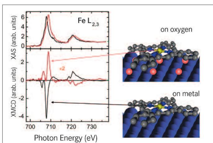
The X-ray absorption spectra (top) are similar for iron porphyrin molecules on nickel with oxygen (red lines) and for nickel (black lines), yet the XMCD difference spectra (bottom) diverge and thereby reveal the antiferromagnetic coupling.
