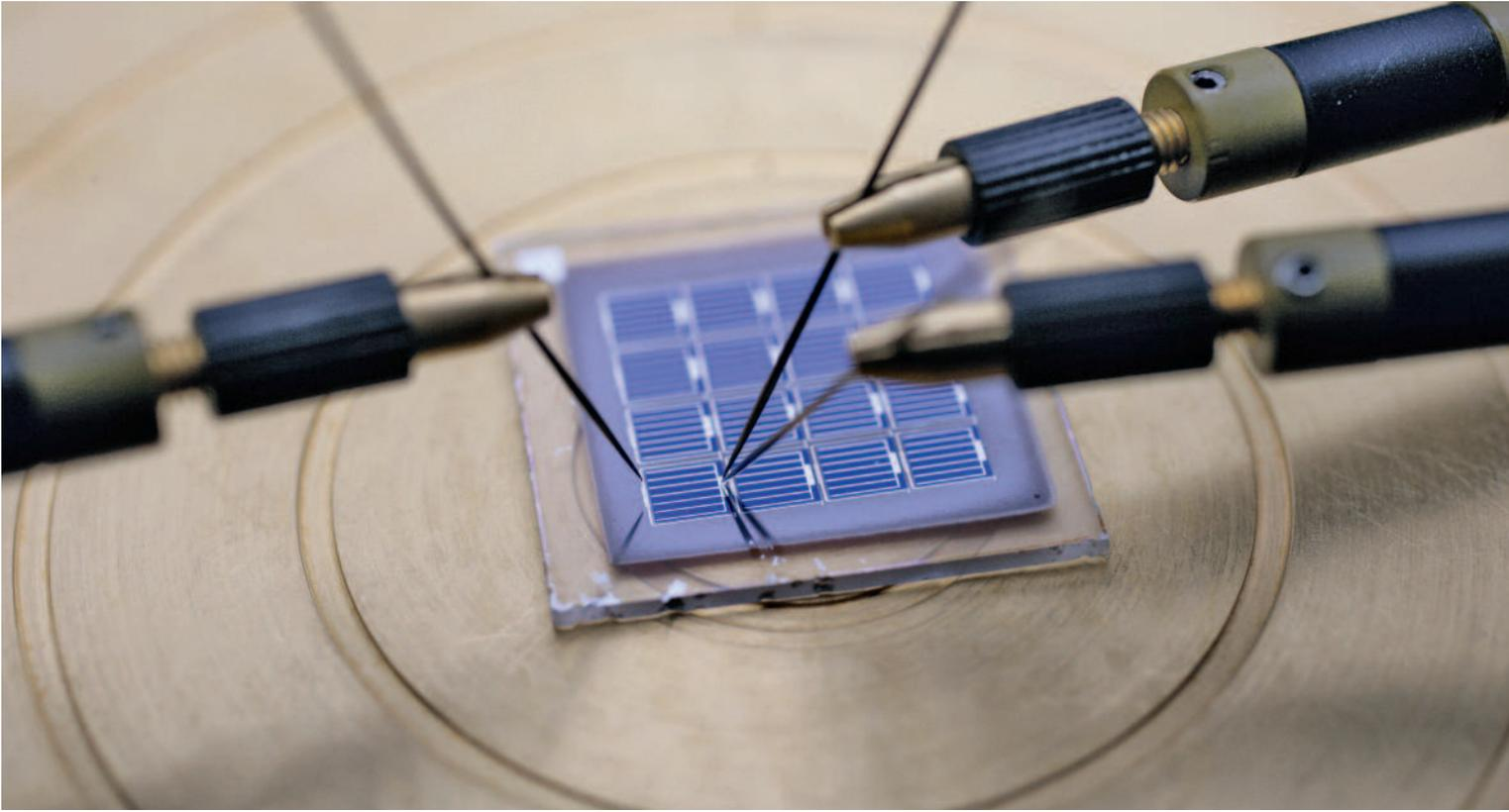
Thin-film solar cells of amorphous silicon as developed by HZB require about 100 times less light-active material (semiconductor) than silicon solar cells.
