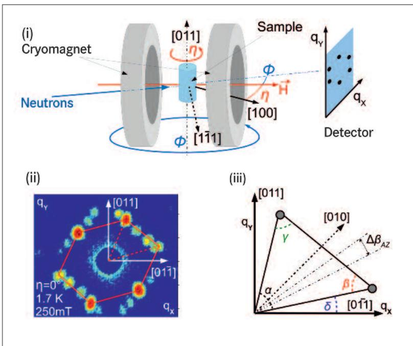
(i) Schematic of Sebastian Mühlbauer and colleagues' setup for measuring flux lattice symmetry, where a sample inside a magnetic field is irradiated with neutrons. (ii) A typical scattering pattern of the flux lattice. (iii) Geometric description of the symmetry of the flux lattice with angle calculations.
