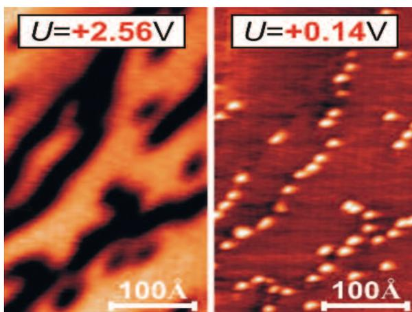
Micrographs of a graphene layer on a nickel substrate. In the image at left, only dark stripes can be seen. Only by cleverly adjusting the photoelectron spectroscopy is it revealed that fullerenes inserted under the graphene layer, that is  $C_{60}$  molecules, are the cause of the striped pattern.
