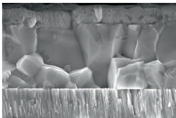
Scanning-electron-microscope image of the layered structures of a CIGSe solar cell.
