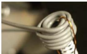
Fig. 1. Photograph of a coil, which produced an alternating magnetic field. 10 A current was varied with frequency of 3 kHz.
