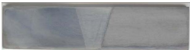
Figure 1 Macrograph of bi-metallic piping weld for investigations.
