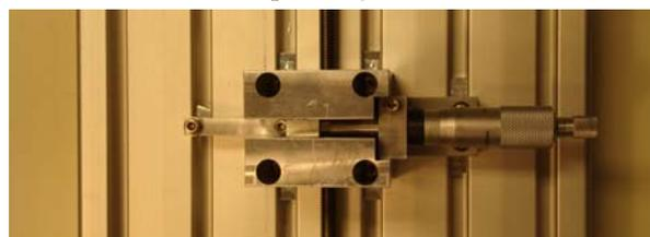
Figure 1: Sample compression stage with possibility of applying a magnetic field of 0.7 T and measuring deformations with an accuracy of 0.01 mm without applying torsion on the sample.
