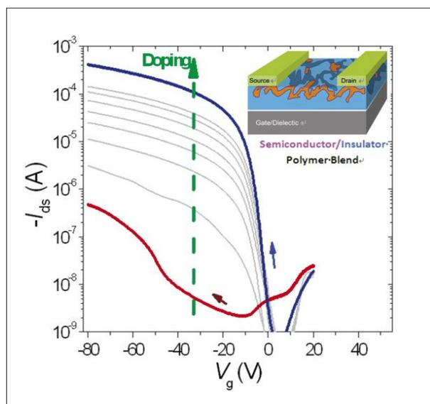
The curve shows how, with increased doping in the semiconductor layer, the transistor ratio improves radically. The researchers ascribe this to the formation of conductive percolation pathways that facilitate the transport of charges along the transistor channel.
