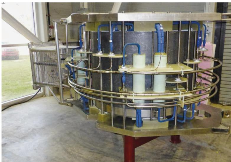
A milestone is reached after five years of developmental work: This is what the new superconductive coil of the new high-field magnet looks like.
