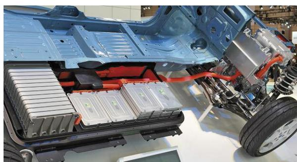
Automobile manufacturers are still using lithium-ion batteries in electric vehicles such as this Nissan Leaf, but research is going full steam ahead in pursuit of better alternatives - not least through experiments at HZB.
