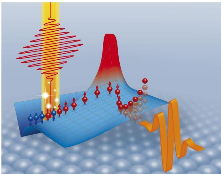
Excited by a femtosecond laser pulse (yellow), an ultrafast spin current occurs (red balls with arrow). It generates electromagnetic radiation in the terahertz frequency range (orange).
