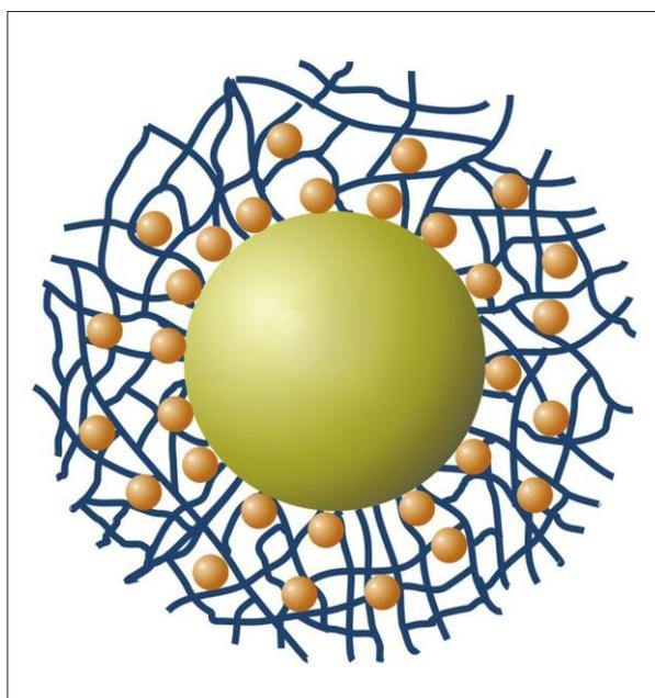
Crystalline titanium dioxide particles about 6 nanometres in diameter form out of solution in the polymer network around the polystyrene core (PS), even at room temperature.
