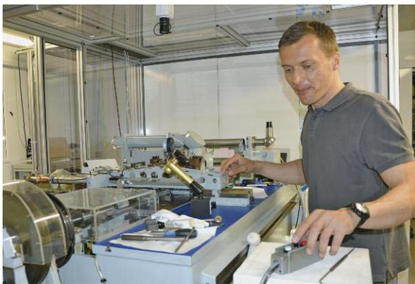
The sawtooth structures are created in this machine. A diamond rules the tiniest of grooves into the gold-coated silicon substrate.
