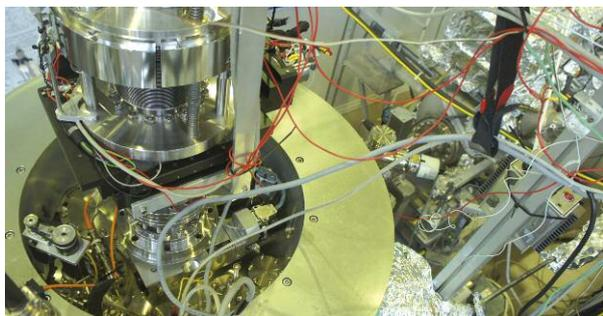
The researchers performed their experiments with lanthanum nickel oxide on the XUV diffractometer developed by HZB.
