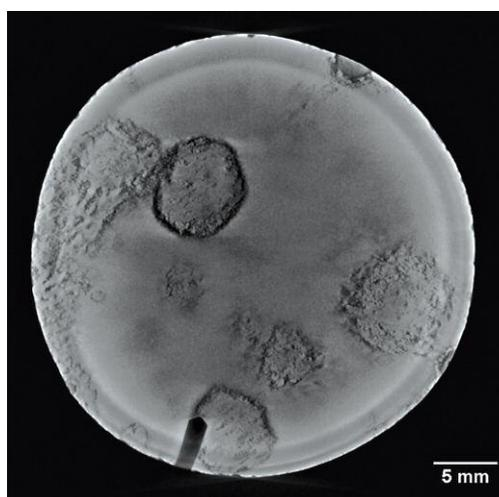
2D X-ray computer tomogram of the Tiberius sesterce taken from the collection in the Duke Anton Ulrich Museum in Braunschweig. Shown is the core of the coin with the drilled hole hailing from an earlier analysis (bottom left) as well as two points of zinc depletion (round surfaces).
