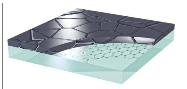
The graphene layer is only one atom layer thick (0.3 ångströms or 0.03 nanometres), yet its charge carriers can move with extreme freedom within it. These properties remain unchanged even when the graphene layer is coated with amorphous or polycrystalline silicon.
