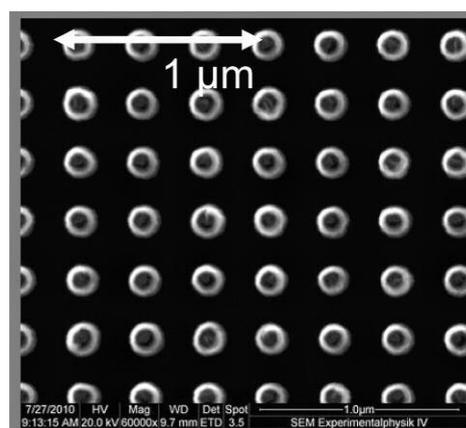
Scanning electron micrograph of a regularly arranged square lattice made up of magnetic islands. The researchers revealed the islands by means of electron beam lithography.
