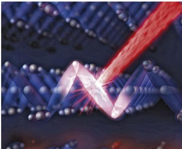
An optical laser flash (red) disrupts the electronic order (blue) in magnetite, switching the material's state from insulating to conducting within a trillionth of a second.
