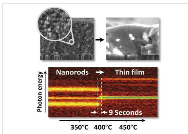
The transition from a layer of densely packed nanorods (top left) into a polycrystalline semiconductor thin film (top right) can be observed in realtime using in-situ X-ray diffraction. In the bottom image, the intensity of the X-ray signals is colour-coded. Detailed analysis of the signals reveals that the transformation from nanorods to kesterite crystals takes only 9 to 18 seconds.
