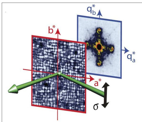
Stripe pattern of charge carriers in  $\text{Bi}_2\text{Sr}_2\text{CaCu}_2\text{O}_{8-x}$ . The figure shows the structure with a period of about one nanometre (front) and the associated diffraction pattern (back) in the form of a so-called Fourier transformation.
