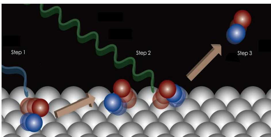
First, the CO molecules were detached from the crystalline surface of the ruthenium catalyst using conventional laser pulses (blue), after which the researchers could observe using X-ray pulses on the LCLS (green) that these molecules remain close to the surface over a substantial period of time and can only move parallel to it. Only after a certain time (step 3) do the CO molecules completely escape from the surface.
