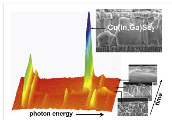
Growth of the layers can be analysed using in-situ X-ray scattering and fluorescence signals.
