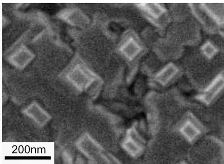
Scanning electron micrograph of the barium titanate layer in which the tiny pillars of cobalt ferrite measuring only a few nanometres are embedded.
