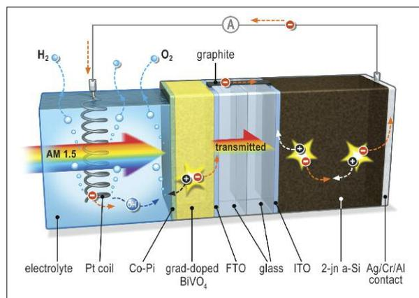
When light strikes the system, an electric voltage is created. The metal oxide layer acts as a photoanode, where oxygen forms. It is connected to the solar cell via a conductive graphite bridge (black). Because only the metal oxide layer comes into contact with the electrolytes, the rest of the solar cell remains protected against corrosion. A platinum coil serves as a cathode, where hydrogen forms.
