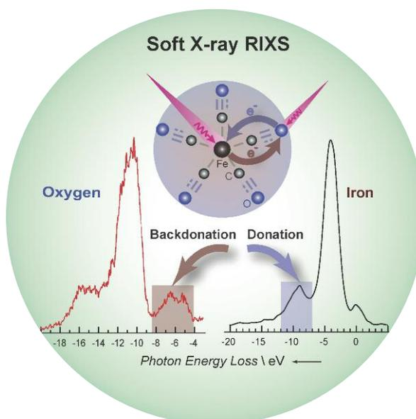
Elementary processes in the limelight: Donor and acceptor binding properties of the model catalyst  $\text{Fe}(\text{CO})_5$  in solution are studied by resonant inelastic X-ray scattering.
