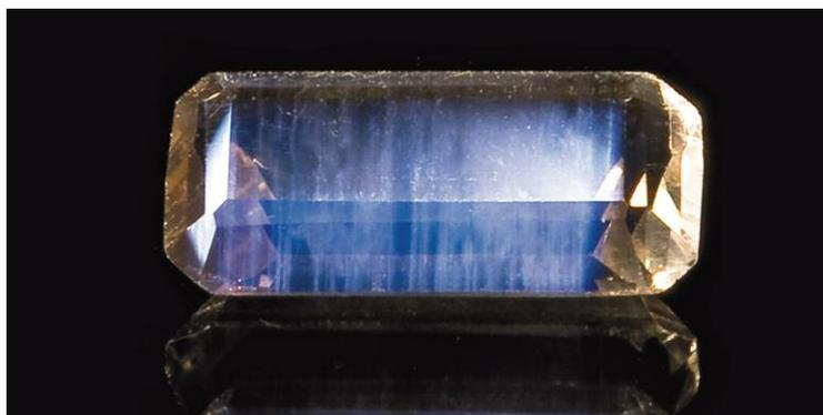
Blue sanidine variety. After a while, the crystals display defects that can be “healed” with high temperatures. HZB researcher Johannes Kähn investigated exactly what happens during the process.
