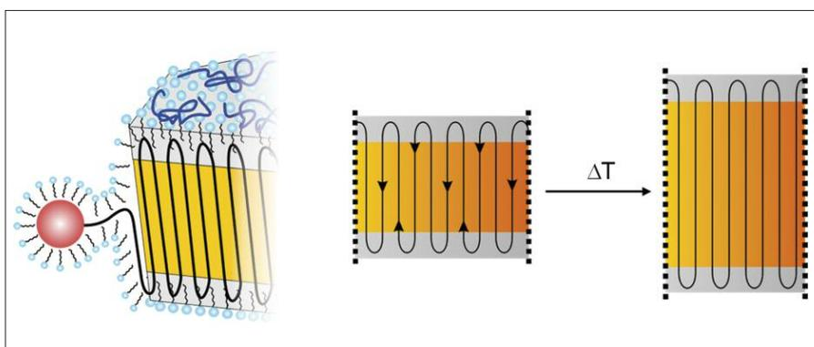
A water-soluble Ni(II) catalyst allows the polymerization of ethylene in aqueous solution. The illustration shows how the newly created parts of the PE chain are incorporated into the growing crystal. The amorphous areas act in the ideal nanocrystal like deflection pulleys that reverse the direction of the chains by 180 degrees.
