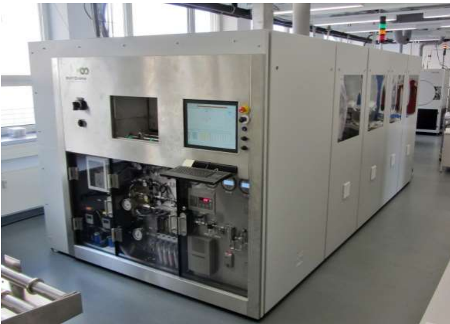
SMIT Thermal Solutions atmospheric chalcogenization in-line machine.
