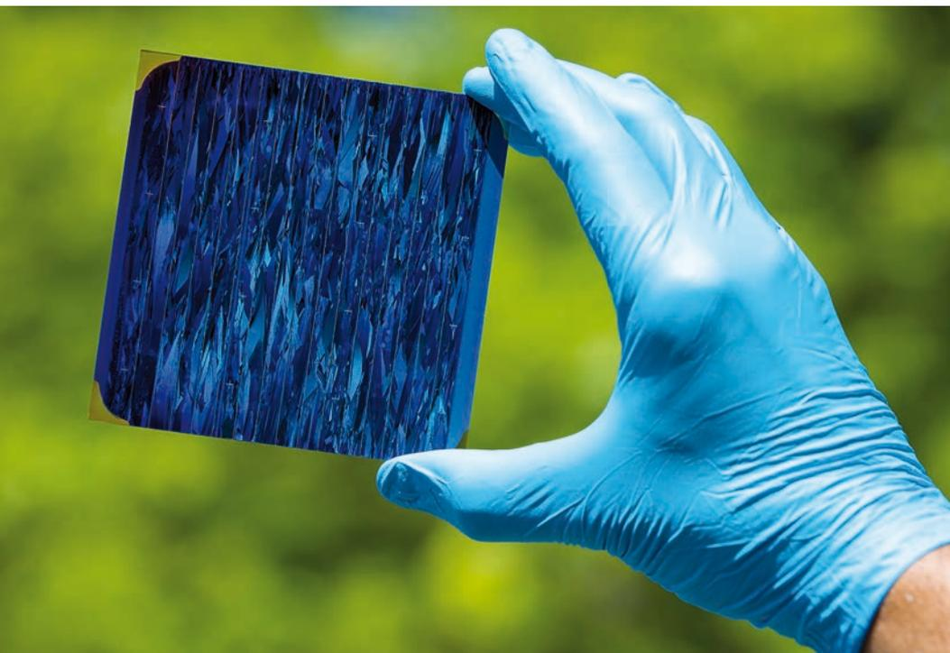
Fig. 4 Si crystal grain structure created by cw line shaped diode laser LPC treatment of a 10  $\mu\text{m}$  Si thin film on 10 cm  $\times$  10 cm glass substrate. (Source: HZB / HySprint)
