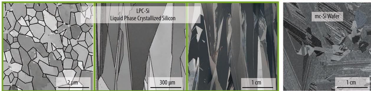
Fig. 3 The green box depicts the flexible grain size tuning achieved with the LPC technology utilizing a line-shaped diode laser. Depending on the crystallization parameters, the grain size ranges across several orders of magnitude and can be tuned to fit the desired requirements (left). A micrograph of a multi-crystalline Si (mc-Si) wafer is depicted in the grey box for comparison (right; Source: HZB / HySprint).
