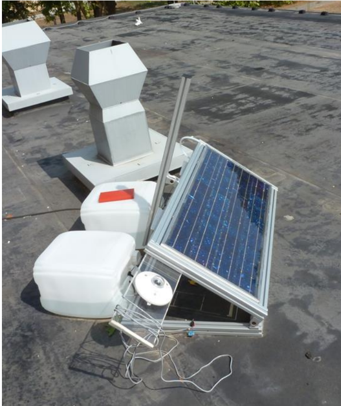
Figure 5: PV panel and pyranometer combined with PEM electrolysis on the rooftop of IEK-3 at Forschungszentrum Jülich.
