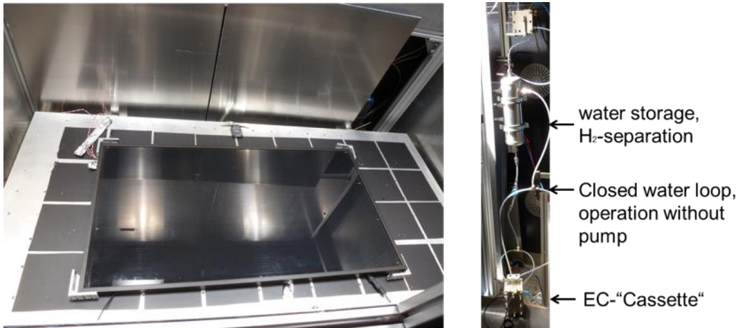
Sun simulator with PV solibro module (630x1190mm; 0.75m 2 )
