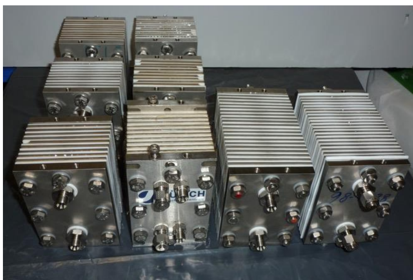
Figure 5. PEM electrolyser stacks that have been produced at Forschungszentrum Jülich GmbH. On the left-hand side are six 10-cell stacks while on the right-hand side, two 21-cell stacks can be seen.
