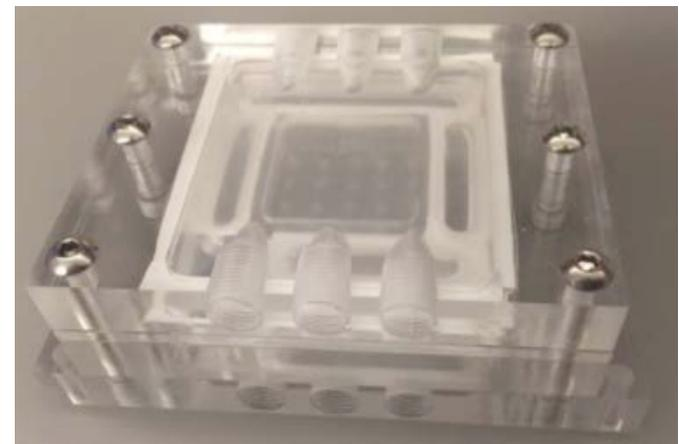
Prototype chassis machined from PMMA
