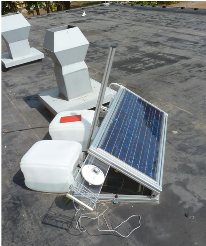
Figure 5: PV panel and pyranometer combined with PEM electrolysis on the rooftop of IEK-3 at Forschungszentrum Jülich.
