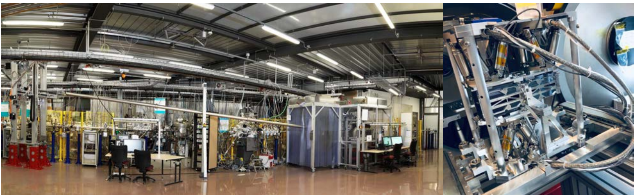
Figure 1: XPBF 2.0 with the sample chamber in a clean tent and the CCD-based detector on a vertical translation with 2 m travel range (left) and hexapod system to align and assemble 4 mirror stacks to a complete mirror module
