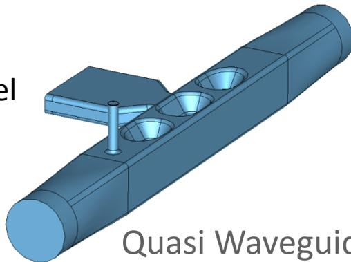
Quasi Waveguide Multicell Resonator
