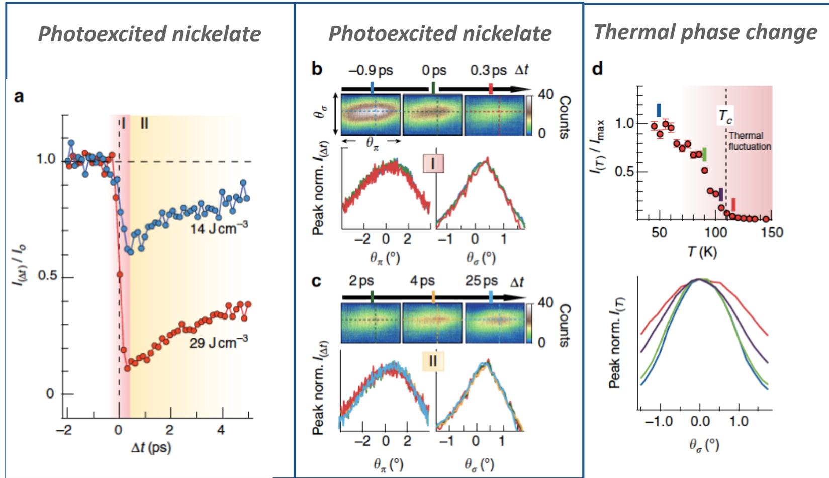
CO recovery timescales measured by XRD:  $\tau_{\text{fast}} = 2$  ps,  $\tau_{\text{slow}} = 57$  ps
