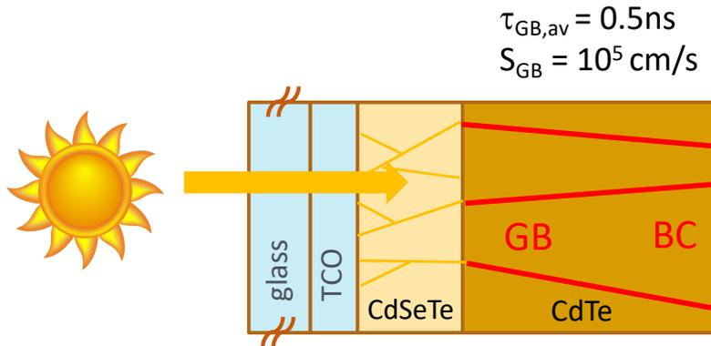
Red lines indicate device areas where recombination reduces carrier lifetimes
