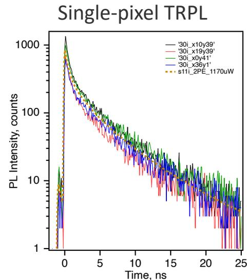
Pixel amplitudes and lifetimes differ with bulk CdTe excitation
