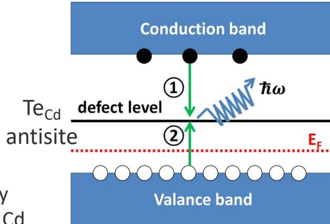
$\text{Te}_{\text{Cd}}$  and  $V_{\text{Cd}}$  density can be changed by Cd partial pressure and CdTe growth temperature:
