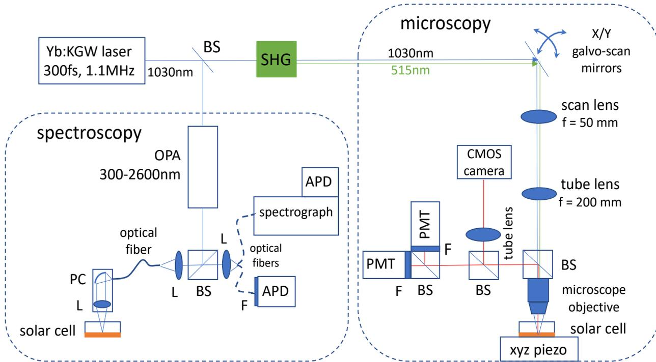
time-resolved laser scanning microscopy with 1030 nm and 515nm excitation
