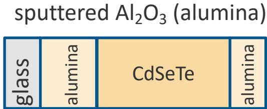
thickness  $d=0.6-4.9 \mu\text{m}$
