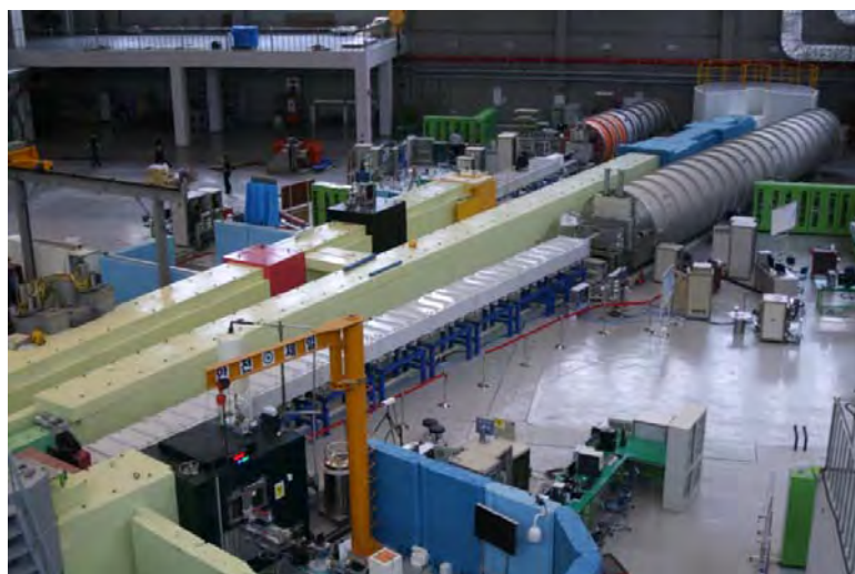
Figure 1: 40m small angle neutron scattering instrument at HANARO.
