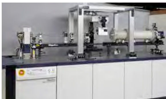
Figure 1: Photograph of 2D SAXS and 2D WAXS simultaneous measurement system.
