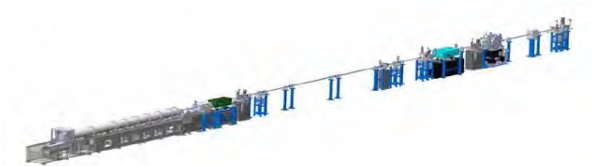
Figure 1: The engineering layout of CXS beamline after front end. On the right (the upstream end of the beamline) are situated a DCM, and a vacuum chamber (in turquoise) housing a set of V-CRLs and the HFM1. On the left are a vacuum chamber (in green) housing a VFM/VDM and the HFM2, and a sample stage. At the end of the beamline is an area detector housed in a 12-meter long vacuum pipe to prevent the signals from being scattered and absorbed by air. (V-CRLs: vertical CRLs; HFM: horizontal FM; VFM: vertical FM; VDM: vertical deflecting mirror)
