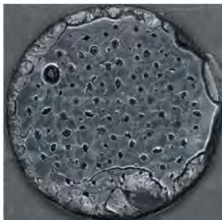
Figure 1: Fracture surface of a SBR-sample with 20 phr CB.
