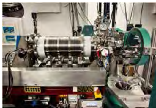
Figure: The moveable detector system (edge welded bellow system) and the sample position of the ASAXS instrument are shown.
