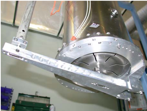
Mechanical tuner with Nb slotted plate (TRIUMF)
