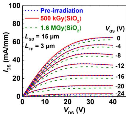
Fig.4: DC output characteristics of field-plated lateral D-mode  $\text{Ga}_2\text{O}_3$  MOSFET before and after gamma-ray irradiations [5].
