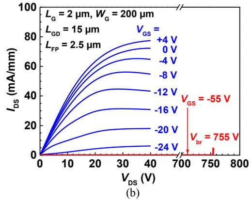
Fig.1: (a) Cross-sectional schematic and (b) DC output characteristics of field-plated lateral D-mode  $\text{Ga}_2\text{O}_3$  MOSFET [2].
