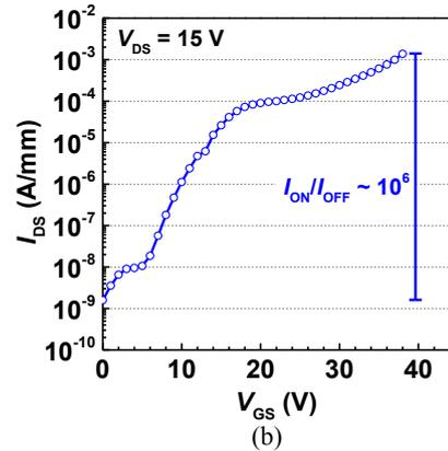
Fig.2: (a) Cross-sectional schematic and (b) DC transfer characteristic of lateral E-mode  $\text{Ga}_2\text{O}_3$  MOSFET [3].
