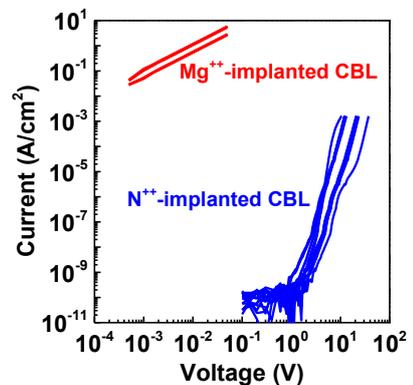
Fig.5: Comparison between leakage currents through N-ion-implanted and Mg-ion-implanted CBLs [6].
