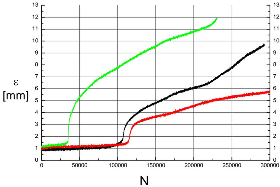
Figure 5: Deformation of AlSi7 foams (density  $0.55\text{g/cm}^3$ ) under cyclic loading with  $\sigma_u = 4.6$  MPa.
