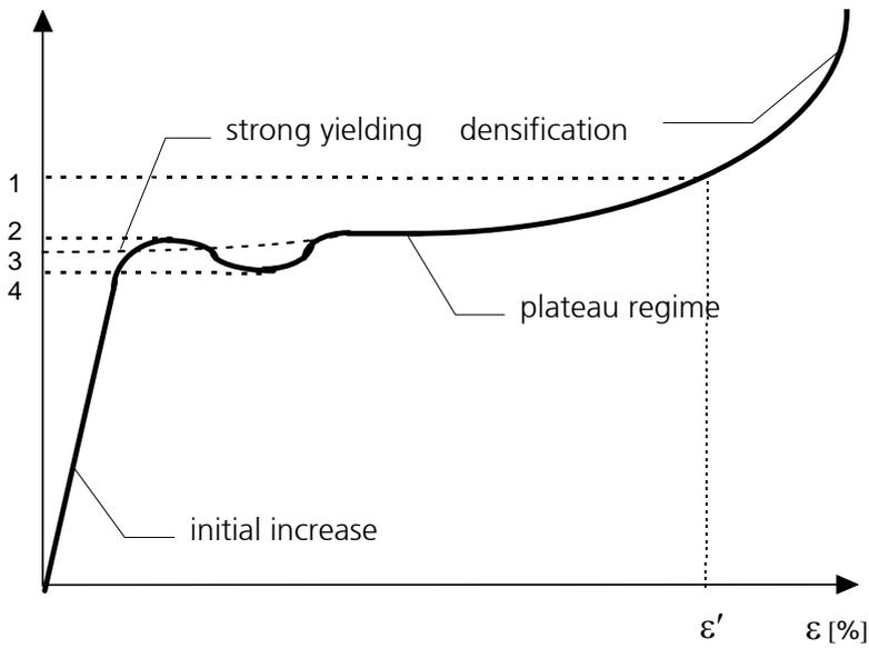
Figure 3: Schematic stress-strain diagram of a foam. The numbers denote the various compression strengths. 1: compression under a given load, 2: upper yield strength, 3: strength extrapolated to  $\epsilon=0$  from the stress-strain curve in the plateau regime, 4: lower yield strength.
