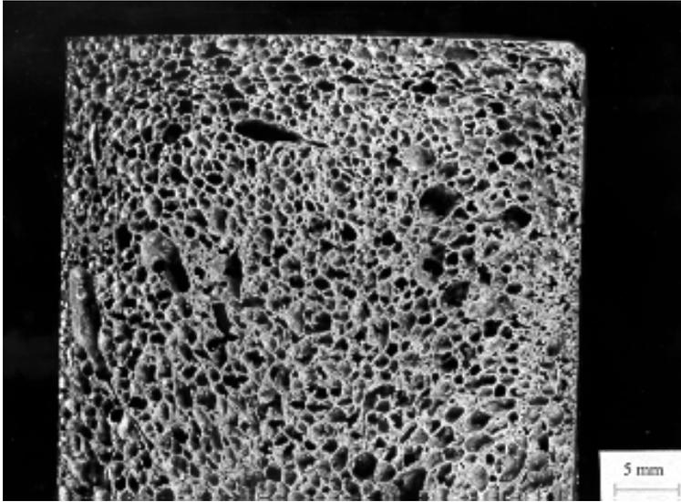
Figure 2: Pore structure of a metal foam sample as shown in Figure 1 (density  $0.55 \text{ g/cm}^3$ ).
