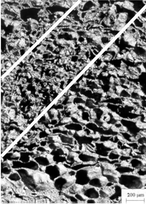
Figure 6: AlSi7 foam after 50% deformation. White lines indicate the boundary of a deformation plane.
