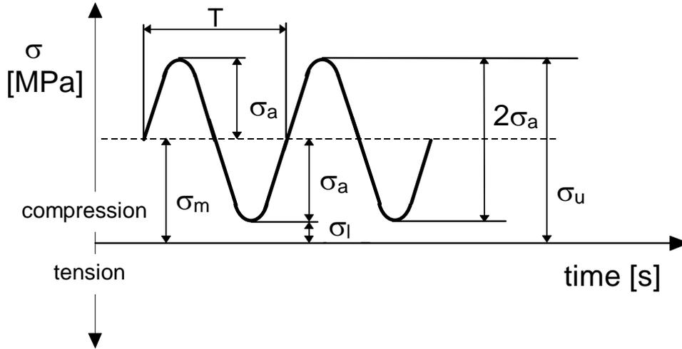
Figure 4: Definition of forces applied in fatigue tests.
