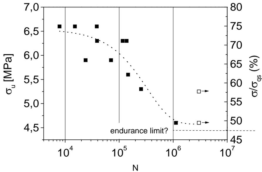
Figure 7: Results of fatigue tests on AlSi7 foams with density 0.63 g/cm<sup>3</sup>. Full squares: <math> < 3 \cdot 10^6 </math> cycles, open squares: no failure after
