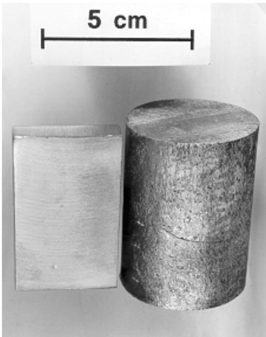
Figure 1: Left: unfoamed aluminium alloy precursor material, right: corresponding foamed part as used for the tests.
