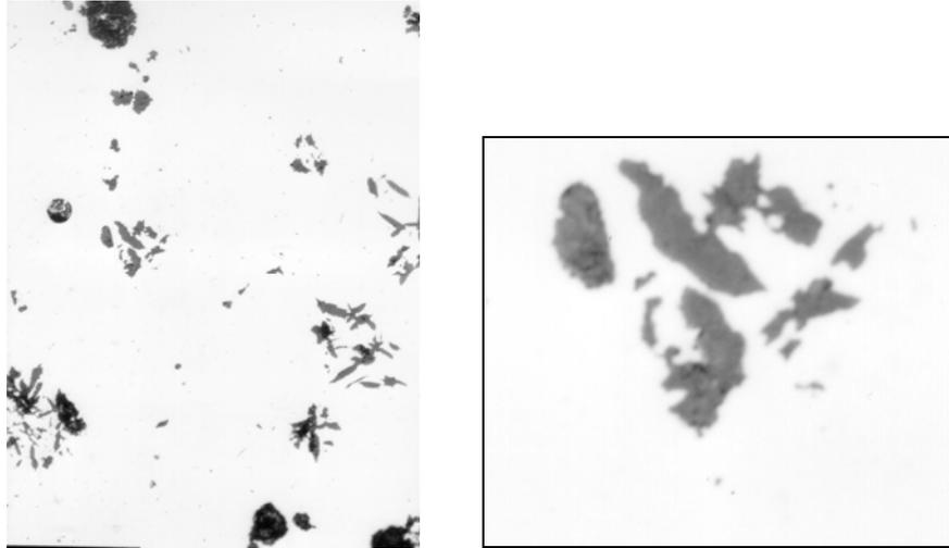
Figure 3: SiC particles embedded in C35 steel (volume content about 4%)
