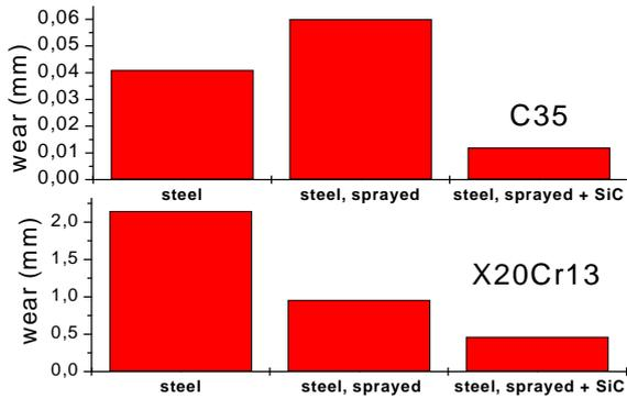
Figure 4: Wear tests on untreated, spray formed and particle-reinforced reinforced steels.
