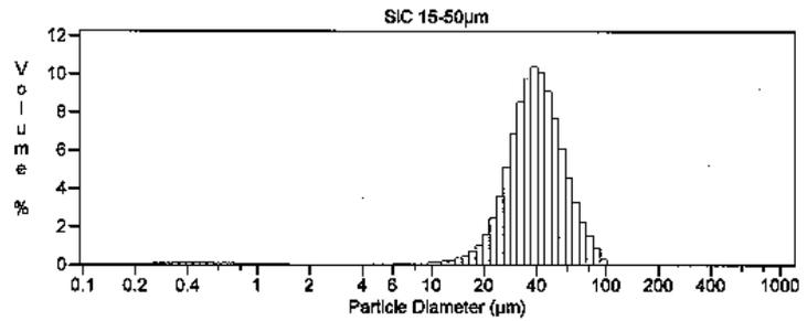
Figure 1: Particle morphology and size distributions of the SiC powder used
