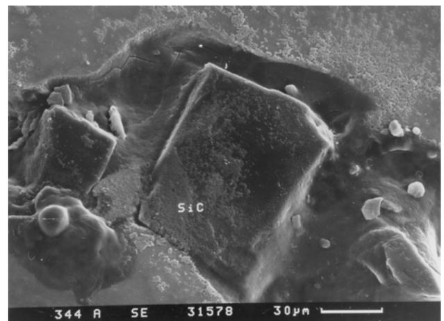
Figure 2: Steel C35 with embedded SiC particles.
