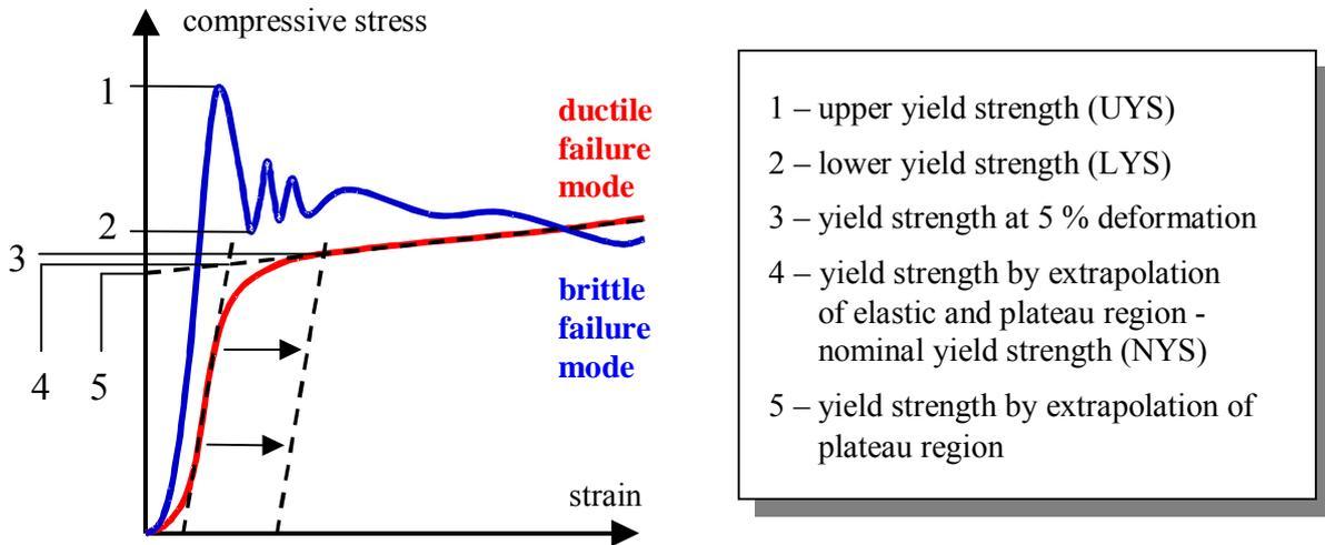
**Figure 1.** Failure modes and common strength definitions for metal foams.
