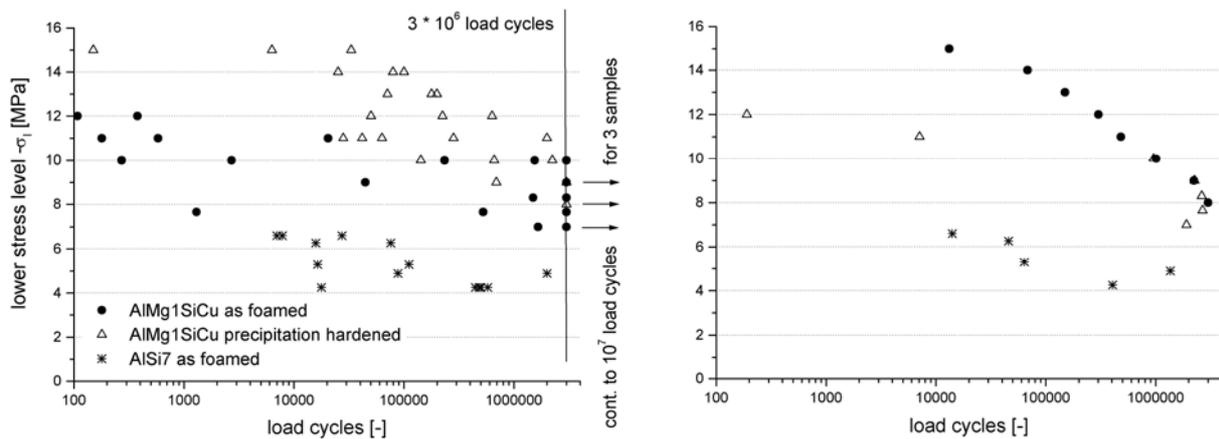
**Figure 4.** Compression-compression S-N curves for AlMg1SiCu alloys in two different heat treatment states. Individual measurements are given in the diagram to the left, in which arrows denote samples that survived further testing to  $10^7$  cycles. Average values derived from the individual measurements are given in the diagram to the right. AlSi7 data is also included.
