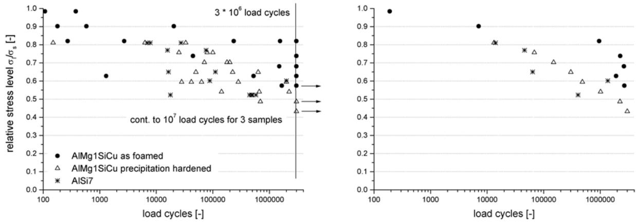
**Figure 5.** Analogous to figure 4. Stresses are given relative to static strength  $\sigma_s$ . Results for AlSi7 alloy foams have also been included.
