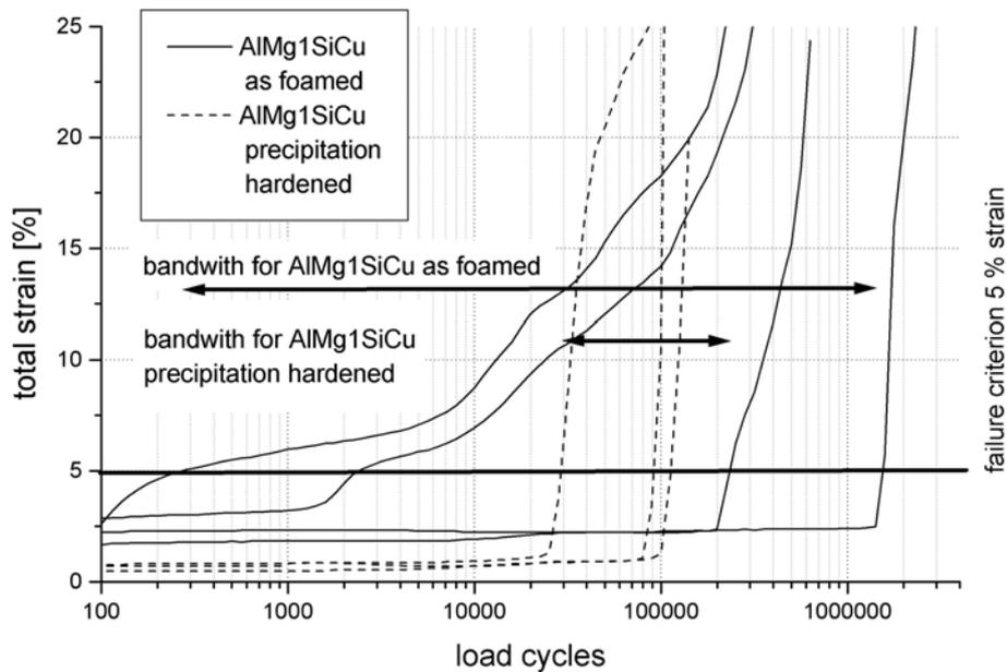
**Figure 6.** Examples of compressive strain versus load cycle curves for individual specimens of the two different types of alloy AlMg1SiCu tested. Stress levels are 10 MPa or  $\sigma_{c,max}/\sigma_s = 0,82$  for AlMg1SiCu without heat treatment and 14 MPa or  $\sigma_{c,max}/\sigma_s = 0,76$  for precipitation hardened AlMg1SiCu.
