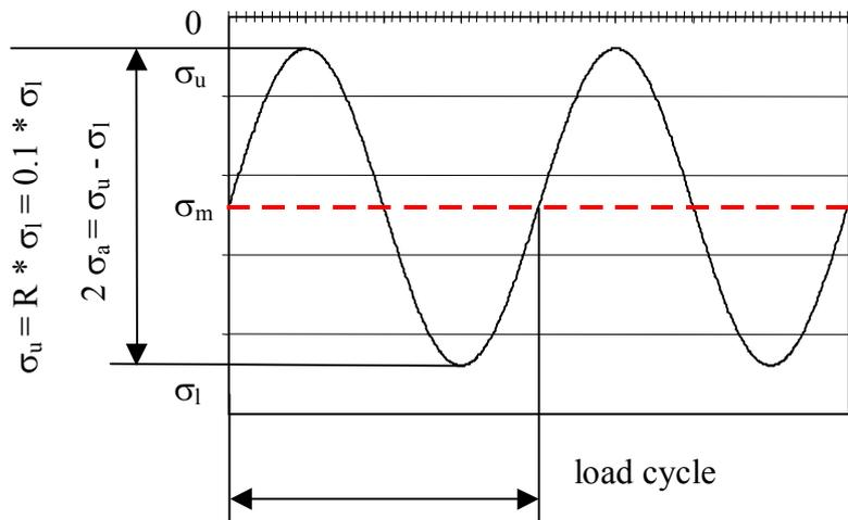
**Figure 2.** Test set-up and general concept of fatigue tests – note that the compressive stress range is examined, for which negative stress values are commonly used.
