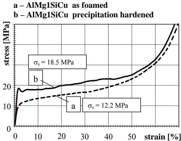
**Figure 3.** Stress-strain curves for as foamed and precipitation hardened AlMg1SiCu foams, density  $0.6 \pm 0.03 \text{ g/cm}^3$  (average of 4 measurements given for each state)
