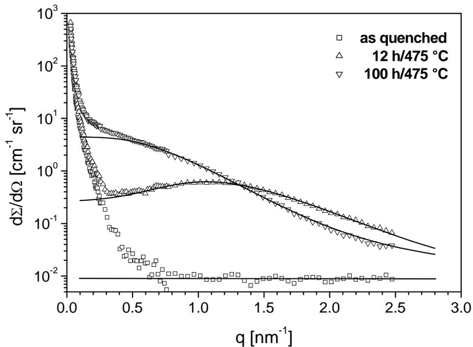
Fig. 4: Magnetic SANS cross-sections of an as-quenched sample and aged samples. Symbols: data; solid lines: fit.
