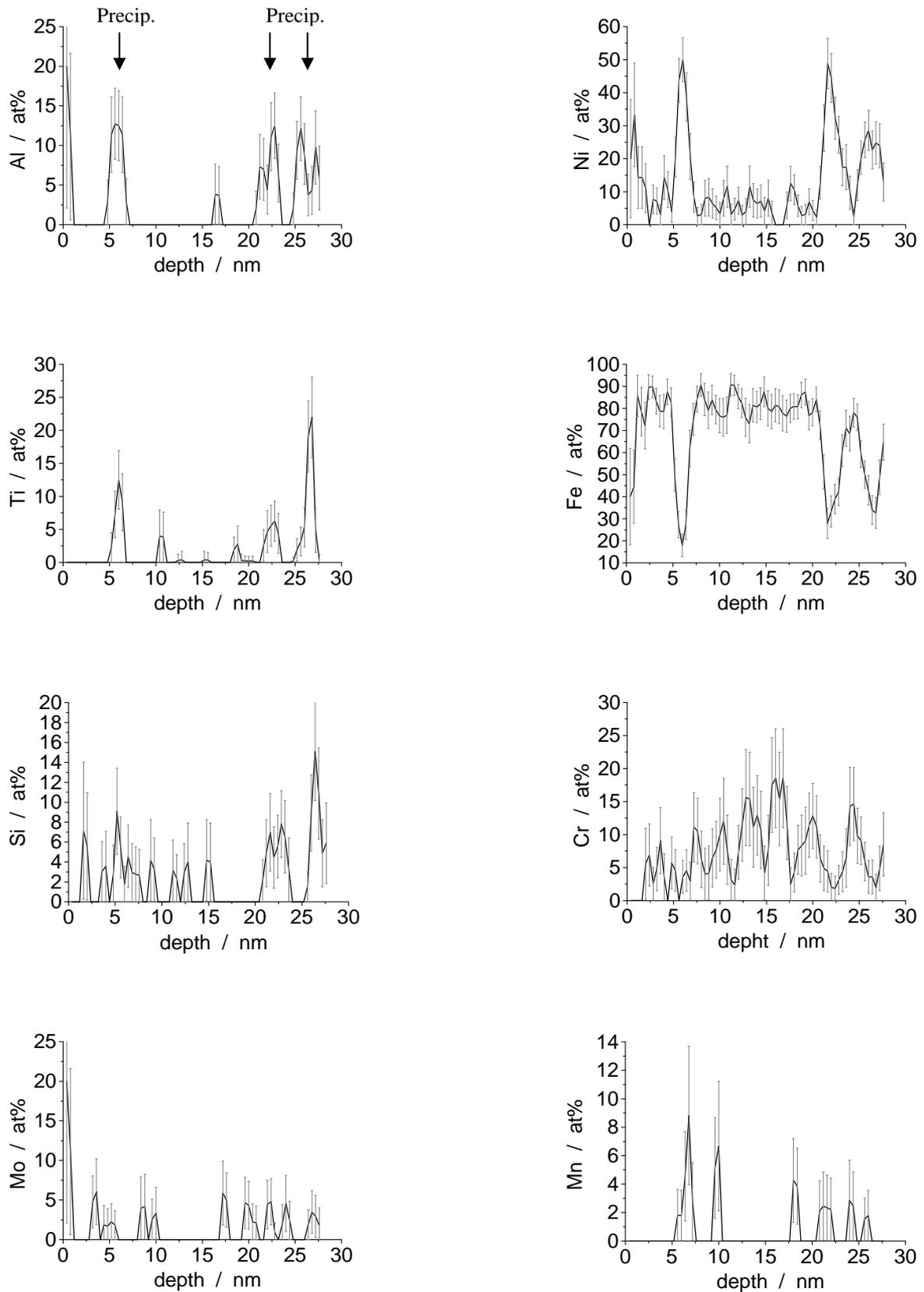
Fig. 2: Concentration depth profiles of the constituting elements (except C) after ageing at 475°C for 12 h. The analysed volume corresponds to the box indicated in Fig. 1a. The arrows denote the position of the analysed particles.
