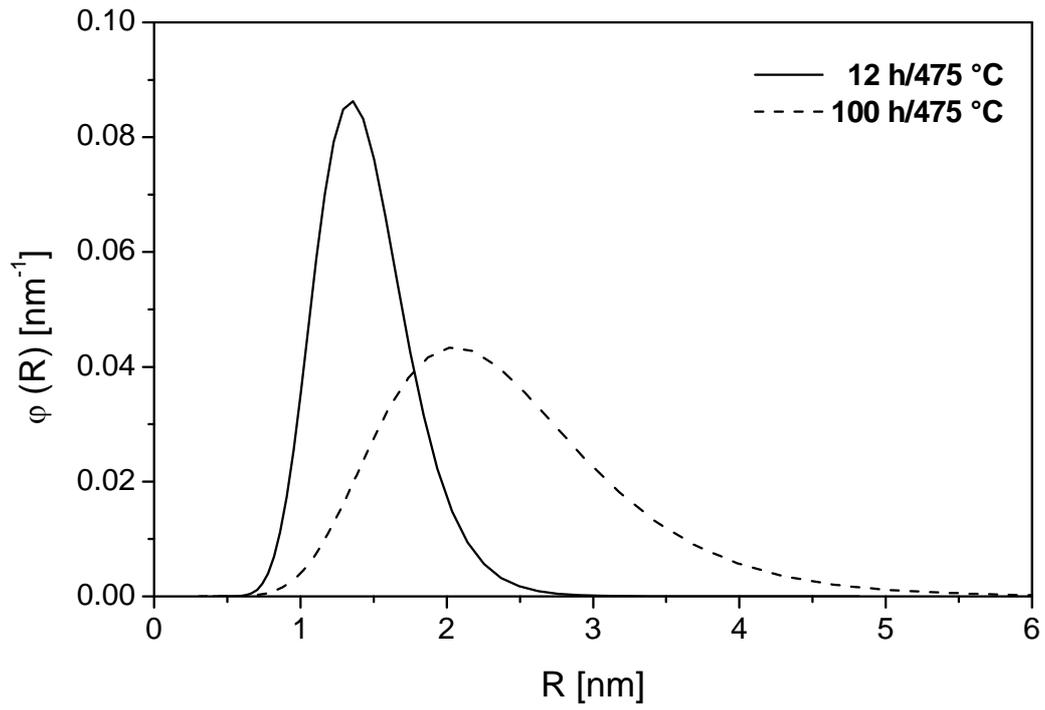
Fig. 5: Particle size distributions obtained from the magnetic SANS cross-section.
