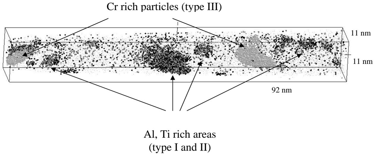
Fig. 3: Three dimensional elemental mapping of Al and Ti atoms within the analysed volume of  $11 \times 11 \times 92 \text{ nm}^3$ . Chromium atoms within clusters with more than 20 at.% Cr concentration are displayed in the same volume.
