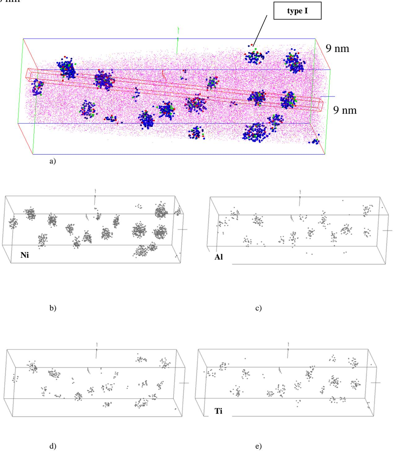
Fig. 1: a) Three-dimensional reconstruction of the position of Ni, Al, Ti, and Si atoms in a volume of  $9 \times 9 \times 28 \text{ nm}^3$  after ageing at  $475^\circ\text{C}$  for 12 h. Agglomeration of atoms in the same volume: b) Ni with a concentration above 20 at.%; c) Al with a concentration above 6 at.%; d) Si with a concentration above 4 at.%; e) Ti with a concentration above 4 at.%.
