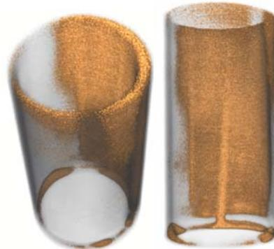
Fig. 5: Neutron tomography of a steel pipe containing some toner of a laser printer and two pencil leads with 0.7 and 0.5 mm in diameter. The toner distribution as well as the pencil leads can be seen.
