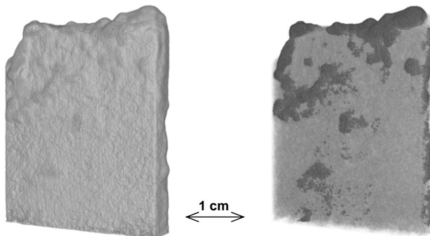
**Fig. 6.** Neutron tomographic reconstruction of a white marble sample from Villa Adriana. a) General view of the sample; b) Visualization of the high-attenuating areas in the sample.
