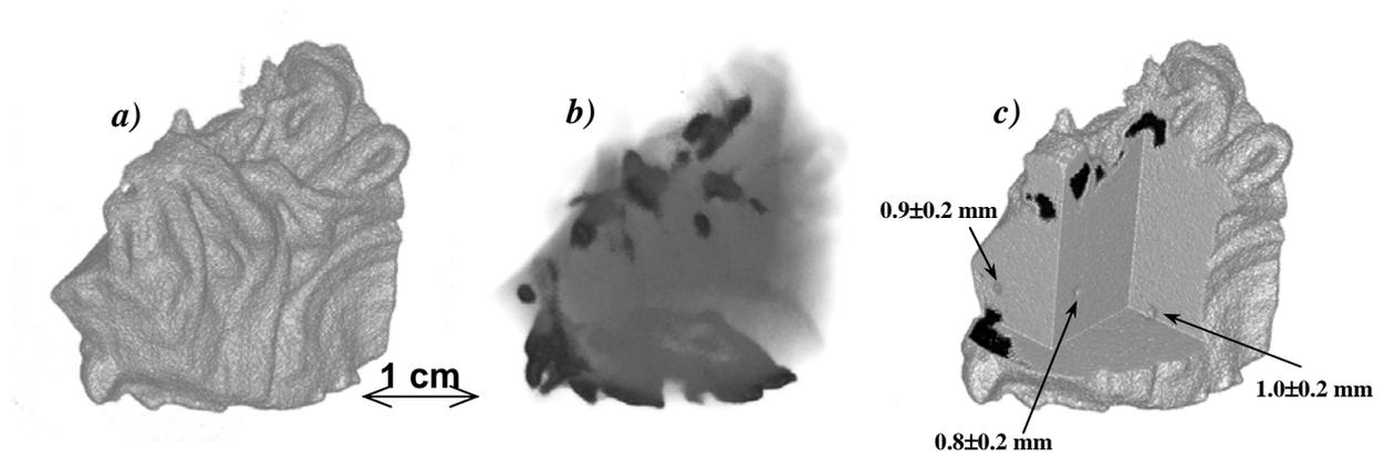
**Fig. 3** Neutron tomographic reconstruction of a glass sample from the excavations in Altino. a) General view of the sample; b) high-absorbing areas; c) quantitative analysis of the voids in the glass material.
