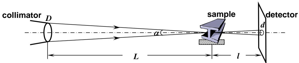
Fig. 2. Schematic representation of a neutron radiographic experimental geometry
