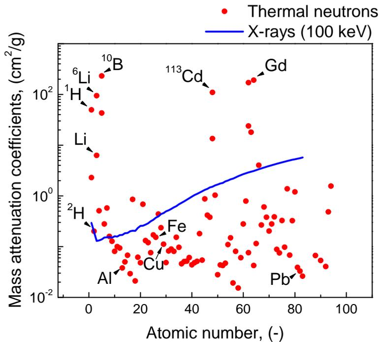
**Fig. 1.** Comparison of the mass attenuation coefficients for thermal neutrons and X-rays (100 keV) in dependence on the atomic number[9].
