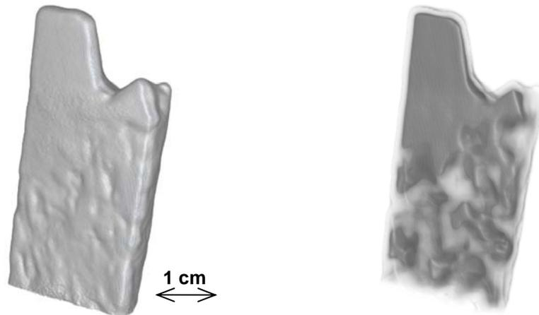
**Fig. 5.** Neutron tomographic reconstruction of a polychromatic marble sample from Villa Adriana. a) General view of the sample; b) Visualization of the high-attenuating areas in the sample.
