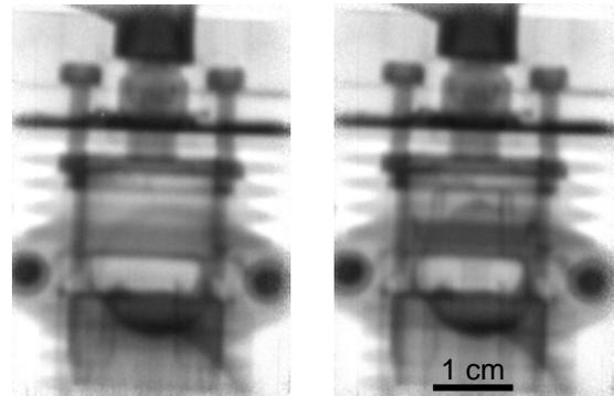
Fig. 3 Two "snapshot" images of the model air-craft engine with a time difference of 5 ms
