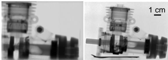
Fig. 5 Model air-craft engine measured at Position I (L/D of 70; exposure time: 0.5 s) and at Position II (L/D of 500; exposure time: 25 s).
