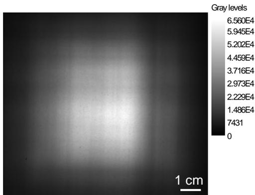
Fig. 4 Beam profile at the measuring position II at the neutron tomography facility CONRAD at HMI.
