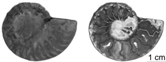
Fig. 6 High resolution neutron tomography of a fossil sample (ammonite). General view (left) and tomography
