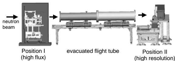
Fig. 2 Drawings of the CONRAD instrument set-up
