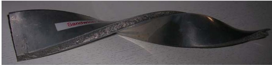
Figure 3. 3D-shaped AFS made by torsional deformation of a strip of AFS precursor, followed by foaming.
