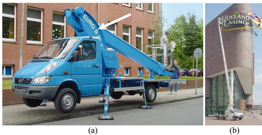
Figure 9. Vehicle with a Teupen 'EURO B25T' lifting arm support. Arrow points at AFS part [67].
