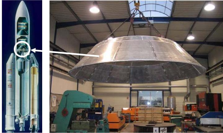
Figure 10. Ariane 5 rocket cone prototype made of AFS [56]. Left image shows location of part in the rocket.
