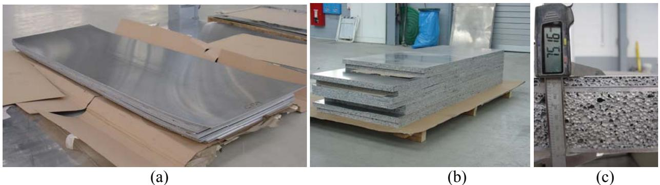
Figure 5. (a) Three-layer composites used for AFS making, (b) foamed AFS panels ready for shipping, (c) comparison of very thin and very thick AFS panel.
