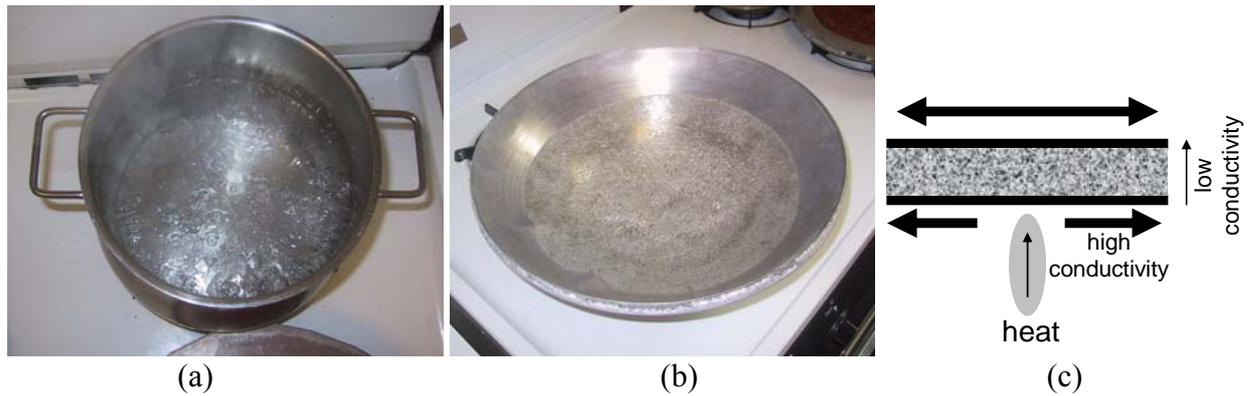
Figure 11. Boiling water in, (a) steel and (b) AFS pan (courtesy of Lisa Smith), (c) thermal flow in AFS pan under cooking conditions.
