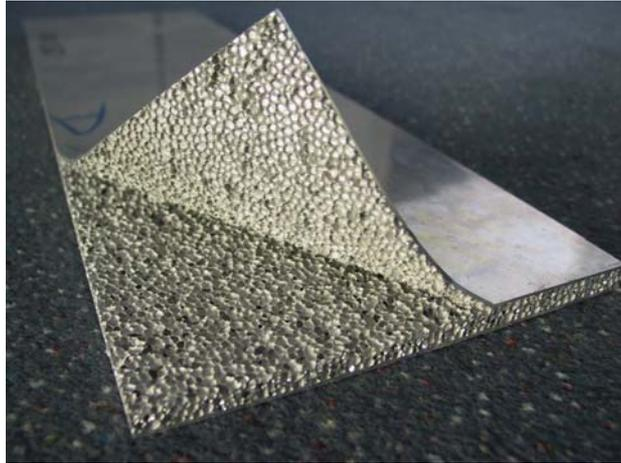
**Figure 3.** Aluminium foam sandwich (AFS) produced by Karmann, Osnabrück (Germany). Face sheet has been peeled off to make the pore structure visible. Note that the strength of bonding between face sheets and foam core is larger than the inherent strength of the foam (courtesy of Karmann).
