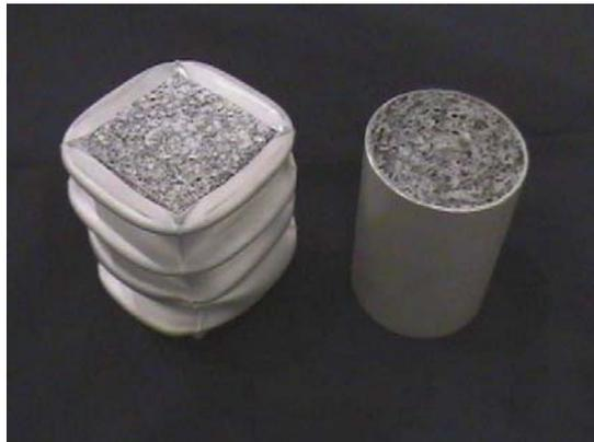
**Figure 4.** Prototypes of crash absorbers based on aluminium extrusions with a filling of Cymat aluminium foam (courtesy of Cymat).
