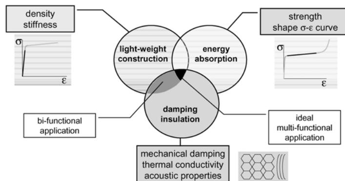
**Figure 2.** Application ranges of metallic foam in automotive industry. Boxes contain the relevant property of the foam which makes it useful for one of the three application fields given in the circles.
