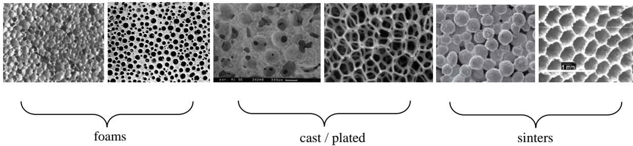
**Figure 1.** Different types of cellular metal. Only the two leftmost structures were foamed in the liquid state: a) aluminium foam, b) copper lotus structure. These are followed by: c) a cast Al sponge made by infiltration of space holders, d) an open cell nickel structure made by coating a polymer foam e) sintered bronze powders and f) a cellular material with oriented pores made by powder metallurgy.
