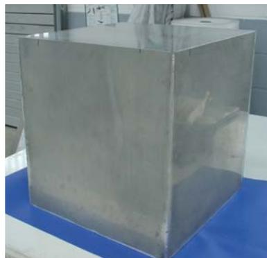
Figure 5. Damping box for electromagnetic waves made of aluminium foam sandwich (AFS).
