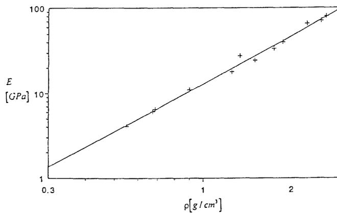
Fig. 3: Young's modulus of AlSi12 foams as a function of the apparent density
