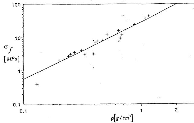
Fig. 2: Compression strength of AlSi12 foams at 20 % deformation as a function of the apparent density
