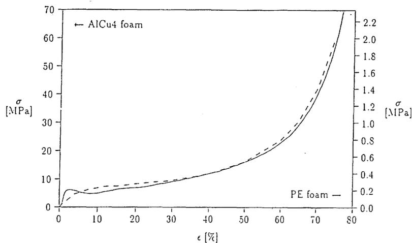
Fig. 1: Compression stress-strain curves of an AlCu4-foam (solid line, left scale) and of a PE-foam (broken line, right scale)
