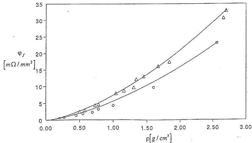
Fig. 4: Electrical conductivity of Al-foams ( $\Delta$ ) and AlSi12Mg-foams (o) as a function of apparent density
