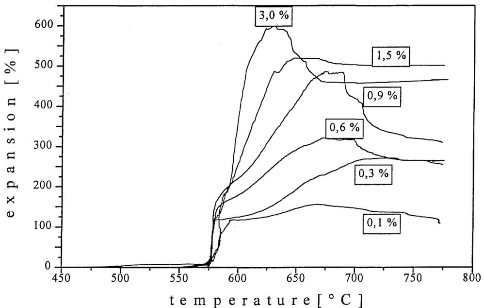
Fig. 3: Comparison of foam expansion (AlSi12) for different foam agent contents
