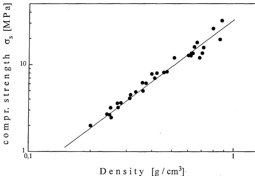
Fig. 1: Compression strength of AlSi12 foams after 20 % deformation
