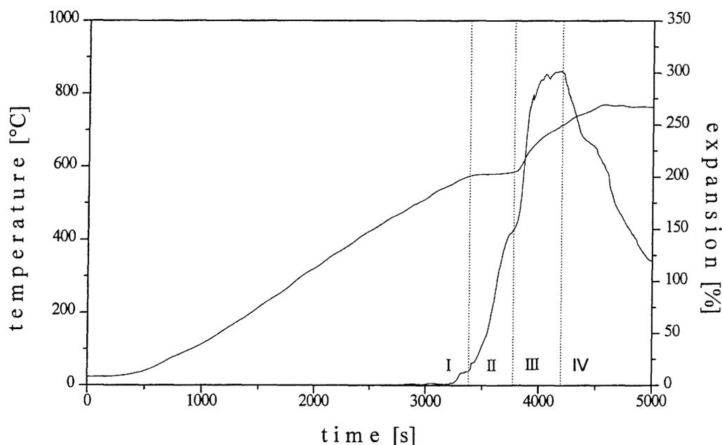
Fig. 2: Expansion characteristics of AlSi12 (heating rate 10 K/min)
