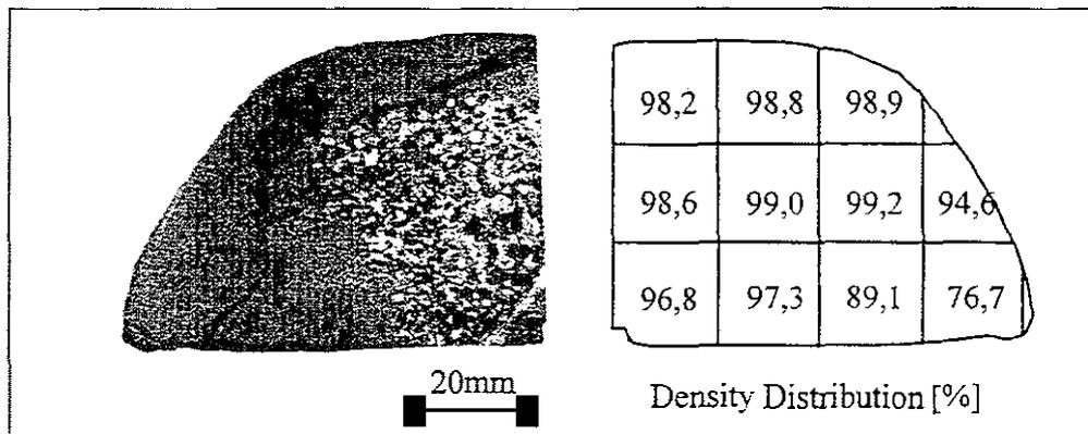
Figure 5. Microstructure development (left) and density distribution (right) of a billet, sprayed with  $\Delta T=350\text{K}$  and  $p=2,5\text{bar}$  ( $\text{GMR}=0.95$ )
