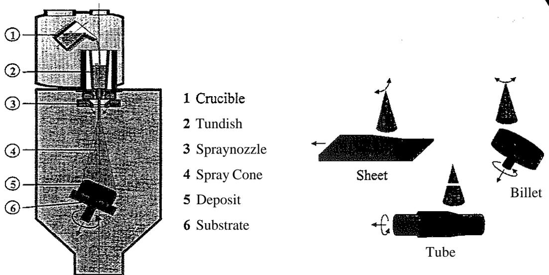
Figure 1. Schematic view of an experimental spray forming facility and of spray formed products
