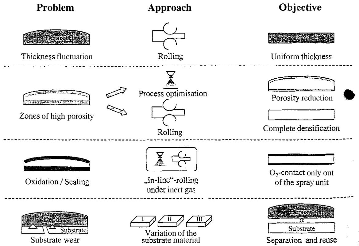
Figure 10. Schematic description of the deficits of spray formed flat products and approaches to quality improvement
