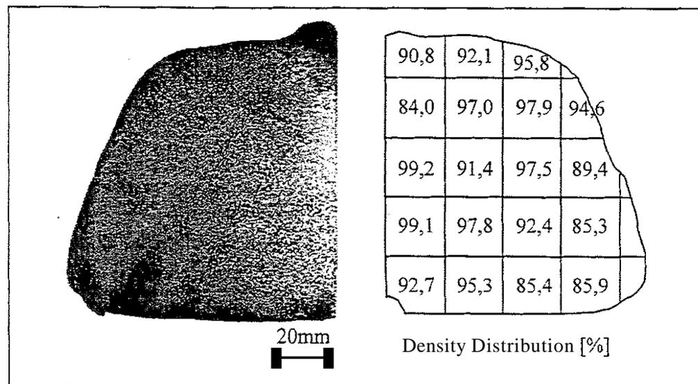
Figure 4. Microstructure development (left) and density distribution (right) of a billet, sprayed with  $\Delta T=300$  K and  $p=2,5$  bar (GMR=0.95)
