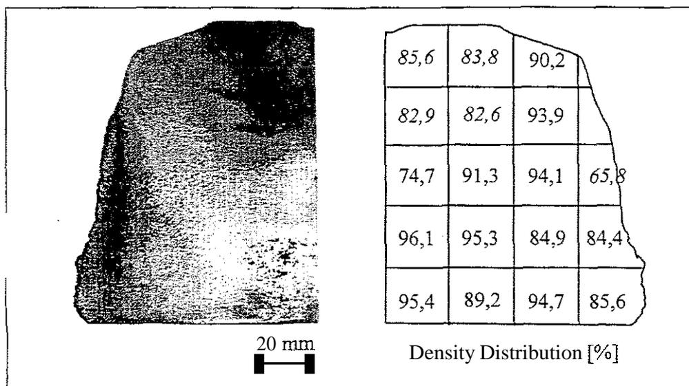
Figure 6. Microstructure development (left) and density distribution (right) of a billet, sprayed with  $\Delta T=300\text{K}$  and  $p=4\text{bar}$  ( $\text{GMR}=1.35$ )
