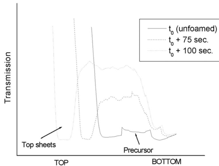
**Figure 5(a):** Transmission X-ray signal – Beginning of foaming
