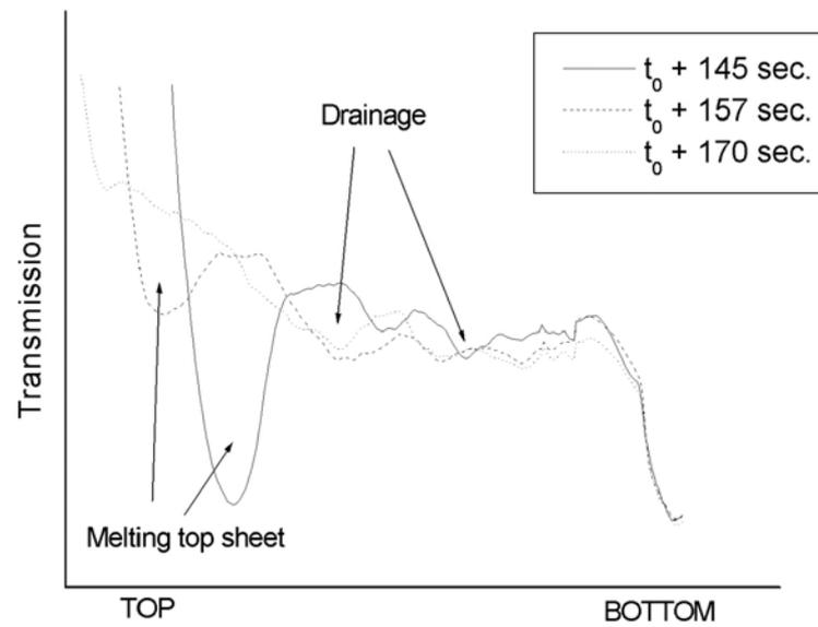
**Figure 5(b):** Transmission X-ray signal - Drainage
