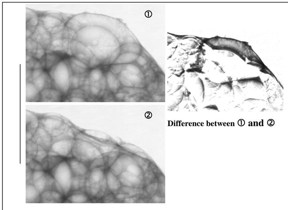
**Figure 4:** An example for cell rupture monitored with X-ray-beam
