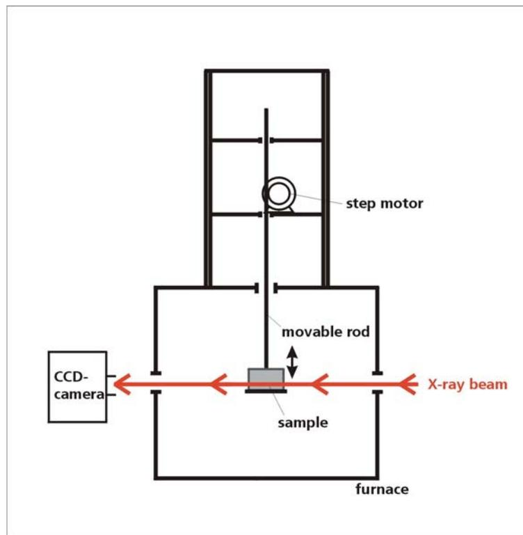
**Figure 3:** Furnace and experimental set-up for in-situ investigations of drainage and cell evolution
