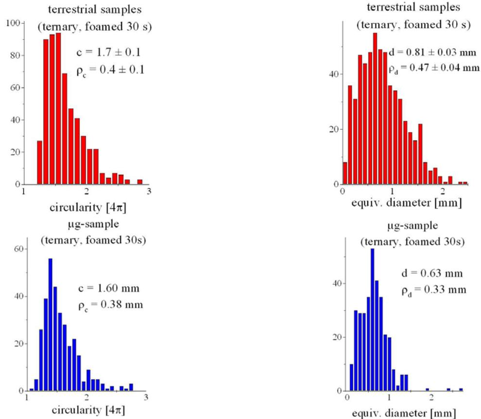
Figure 5: analysis of lead foams manufactured under 1g (upper panel) and “0g” (lower panel). Circularity (left) and equivalent pore diameter distributions are shown [16].
