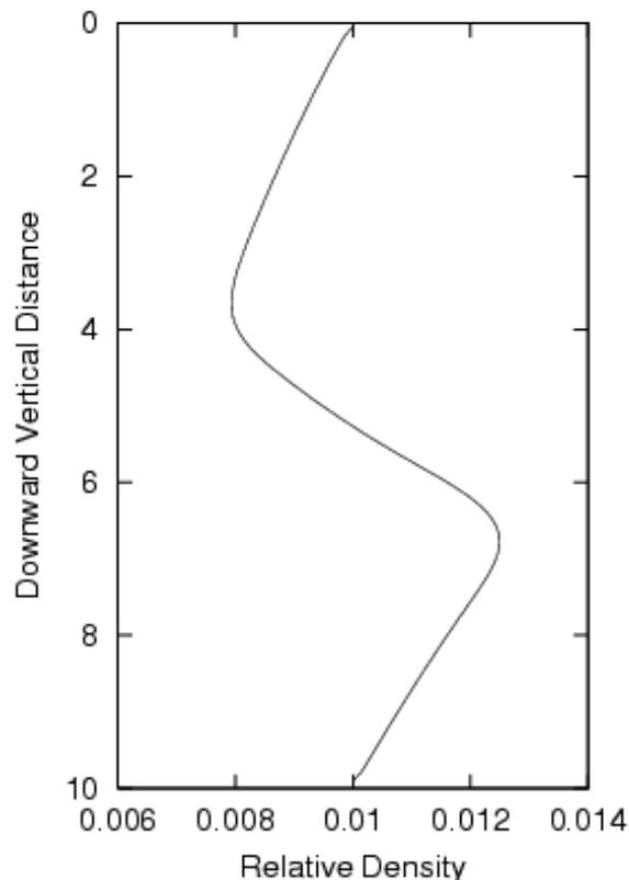
Figure 3: An example of a calculated profile of relative density for an ideal foam which is frozen from the top and bottom. Drainage under gravity induces an inhomogeneous solid product.
