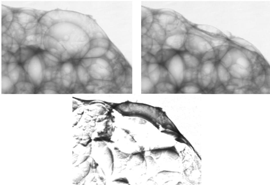
Figure 2: X-ray radioscopic images of an expanding aluminium foam. A series of 900 images was taken with a frequency of 2 per second. Two adjacent pictures and the difference of the pictures is shown. One can see the rupture of an individual cell wall (from [11], see also [12]).
