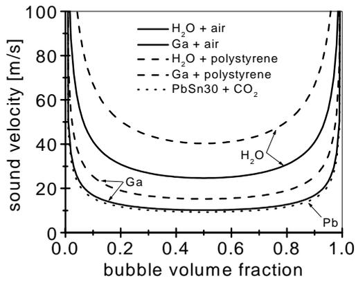
**Figure 1.** Sound velocity for various systems as a function of density.
