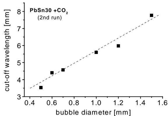
**Figure 4.** Cut-off frequency for various liquid lead foams with various final cell sizes.
