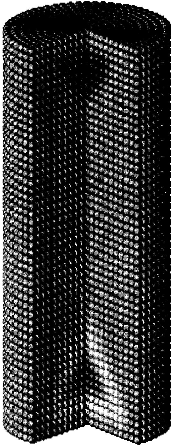
Fig. 5: A cylinder of metallic foam which has been cooled from all sides, and from which a quarter segment has been removed. The coloured spheres denote relative density: the blue areas close to the centre of the top of the sample have low density, while liquid has collected and frozen in the red areas close to the bottom of the sample.
