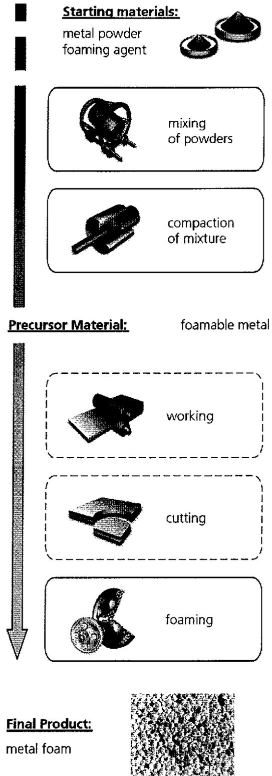
Fig. 1: The powder metallurgical process of metallic foam production.
