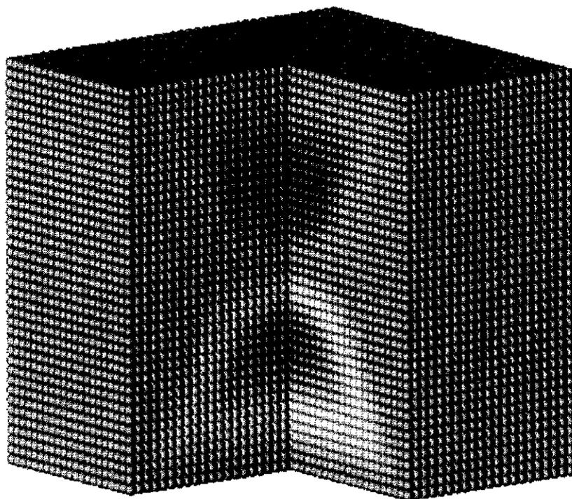
Fig. 6: A cube of solidified foam from which a quarter segment has been removed to show the distribution of relative density. The coloured spheres denote density, as in figure 5.
