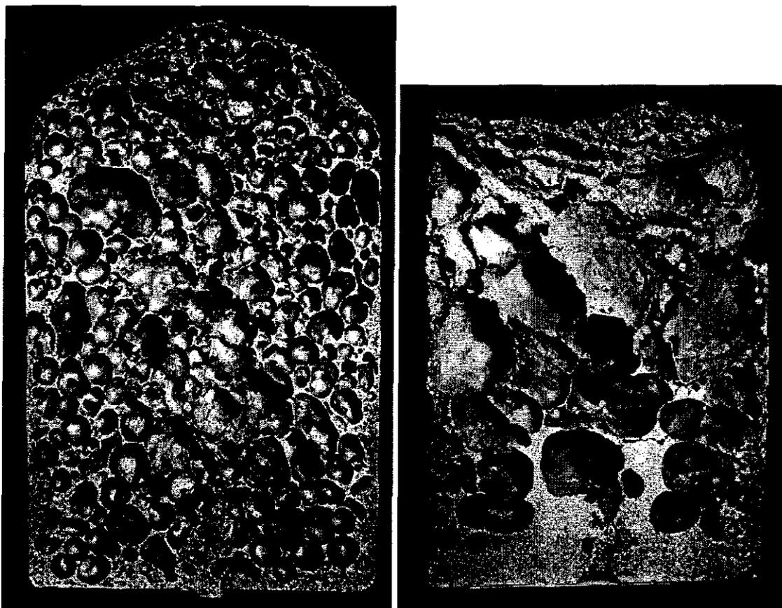
Fig. 2: The photographs show cross-sections through samples of foamed aluminium, which have been formed in a mould. The sample on the left is well-formed, while the one on the right has been kept in the furnace for a longer time leading to structural collapse. Both pictures are reproduced from [1].
