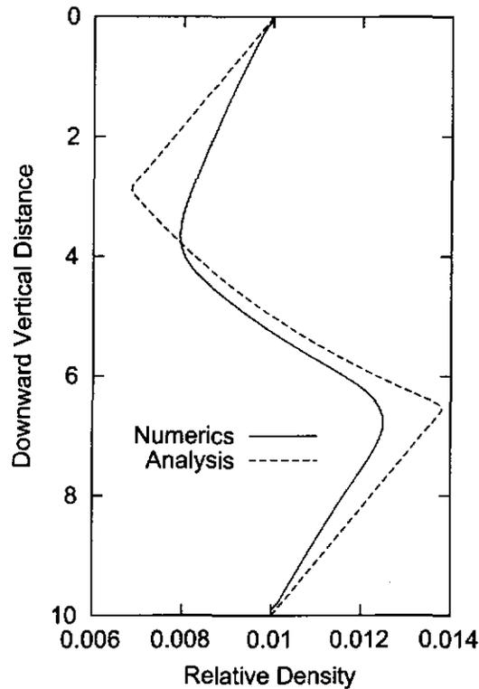
Fig. 4: The final, solidified, profile of relative density in a one-dimensional sample of metallic foam. The numerically obtained profile is compared with a theoretical curve based upon conservation of heat and energy. Both show a decrease in density close to the top of the sample and an increase in density towards the base.
