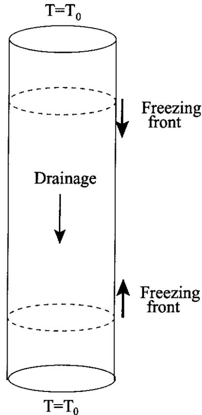
Fig. 3: This sketch of a one-dimensional foam which is cooled from both ends shows that the central region in which drainage occurs shrinks as the freezing fronts move inwards.
