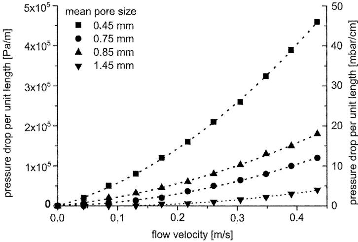
Figure 7.2-2. Pressure drop in partially open-porous cellular solids of the type shown in the middle of Fig. 7.2-1 [8].
