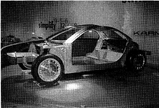
**Figure 3.4-4.** “Detroit Show Car 1998” developed by Karmann (Osnabrück) for demonstrating potential uses of aluminum foam sandwich panels. The rear bulkhead and the front firewall (not directly visible) are made of AFS.
