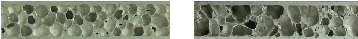
Fig. 1. Aluminium foam sandwich panels. Regular (left) and irregular (right) pore structure.
