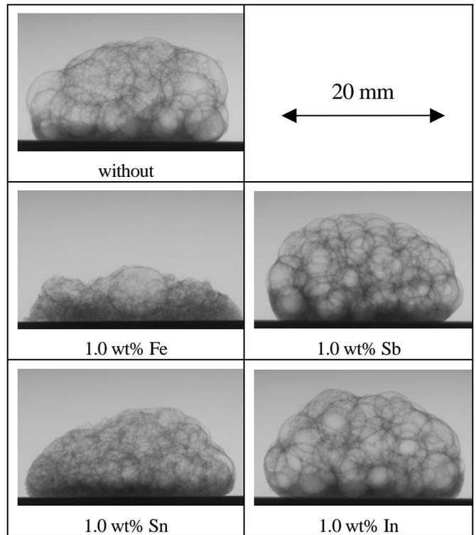
Fig. 8 X-ray radiograms of AlSi11-foams with different additional alloying elements 200s after start of heating, foamed without mould and corresponding to figure 7.
