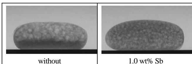
Fig. 10 X-ray radiograms of AlSi11-foams without addition and with 1wt% Sb 75 s after starting heating. Early drainage in the case of no addition can be observed.
