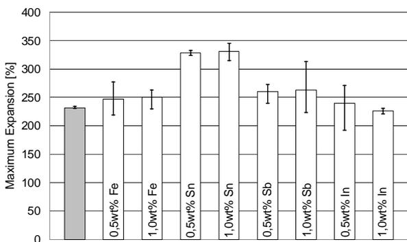
Fig. 4 Average maximum expansion for AlSi11 precursor-material with different additional alloying elements Fe, Sn, Sb and In, T = 750°C
