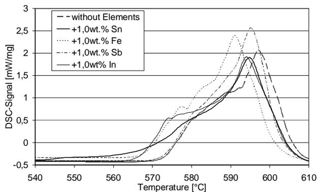
Fig. 12 Influence of the addition of 1wt% of alloying elements on the solidification range (DSC-measurement)
