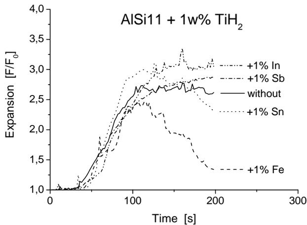
Fig. 7 2D expansion development for AlSi11 precursor material with different additional alloying elements (Fe, Sn, Sb and In),  $T = 700^{\circ}\text{C}$  for  $t > 100\text{s}$
