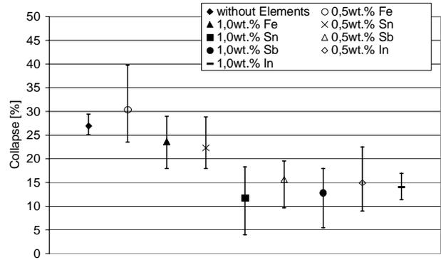
Fig. 5 Influence of alloying elements on the degree of collapse 30 s after the maximum expansion peak, T = 750°C
