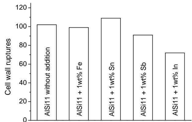
Fig. 11 Coalescence strength quantified by number of cell wall ruptures in fully expanded specimens. Samples correspond to experiment in fig. 7 100s and 200s after the start of heating.
