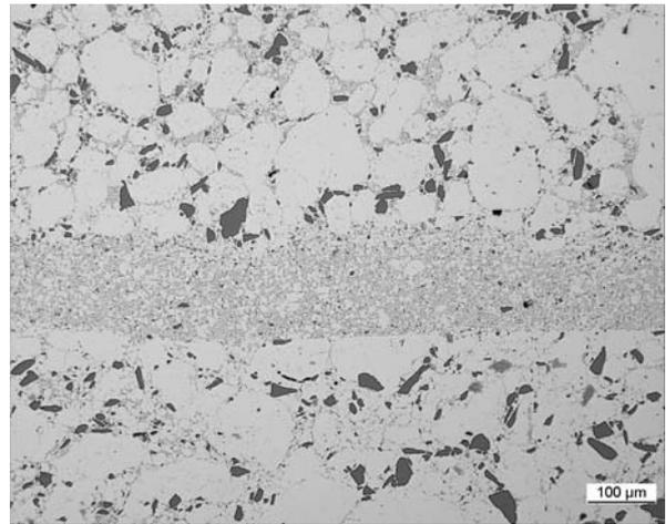
Fig. 1 Metallographic section of the demixing layer rich of eutectic phase near the component surface
