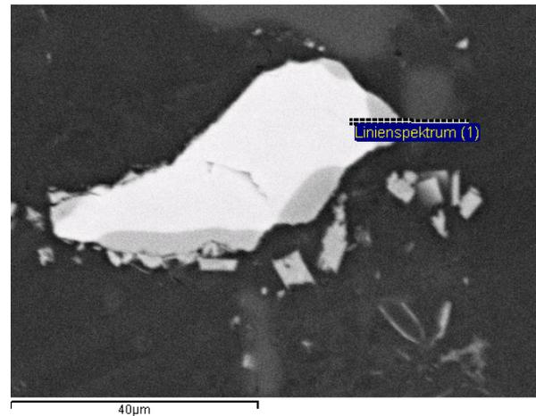
Fig. 2 SEM-figure of a TiH<sub>2</sub>-particle in the as-cast condition of AlSi11-precursor without additions
