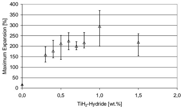
Fig. 3 Maximum expansion of thixocast AlSi11-precursor in dependence of the foaming agent content measured with the mechanical expandometer (minimum, maximum and mean value of 3 specimens), T = 750°C
