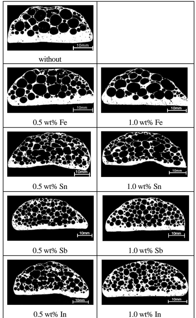
Fig. 6 Pore structure of AlSi11-foams with different additional alloying elements, foamed without mould at T = 750°C.
