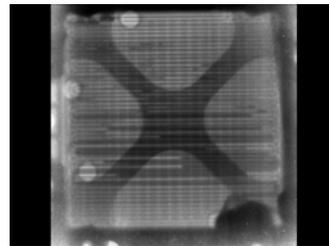
Fig. 2: Radiographic image of a fuel cell. The black horizontal lines are due to the high attenuation of liquid water indicating filled flow field channels.
