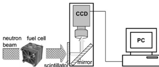
Fig. 1: Schematic drawing of the experimental setup. An almost parallel neutron beam is transmitted through an operating fuel cell to a scintillator screen. The absorbed neutrons produce light spots which are reflected by a mirror detected by a CCD camera.
