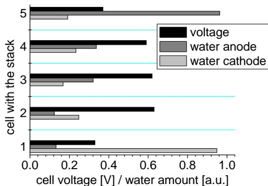
Fig. 4: Water distribution on anodes and cathodes within a 5-fold fuel cell stack compared to the cell voltage. The strong decrease in the cell voltage at the outer cell is due to the flooding of the flow field channels [13].
