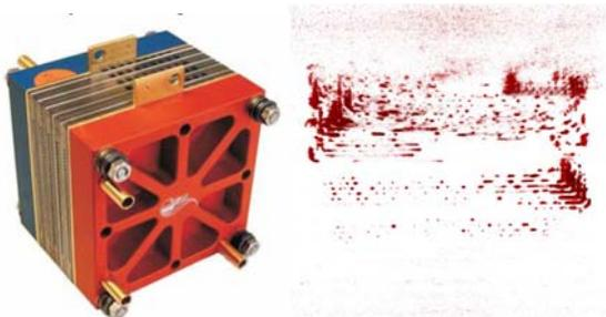
Fig. 3: Left, Photography of a PEM fuel cell stack (right) with dimensions of 14x14x10 cm<sup>3</sup> and a tomographic image of a comparable three fold fuel cell stack (right). All components except the liquid water are turned transparent. This way the three-dimensional distribution of the liquid water can be analysed.
